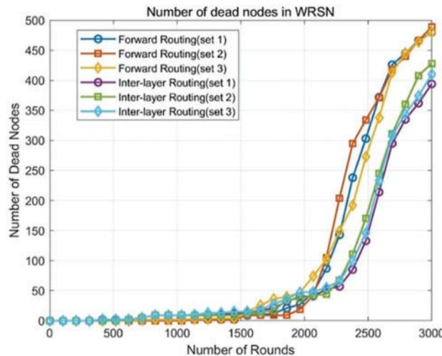
**Figure 5:** Trend of node death in WRSN under two routing mechanisms with different parameters
