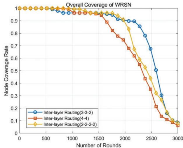
**Figure 13:** Trend of network coverage in WRSN with three different inter-layer relay routing structures
