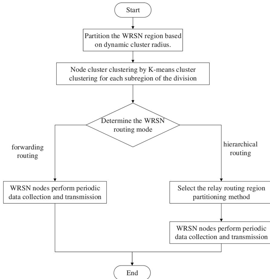
**Figure 4:** Algorithm implementation flowchart
