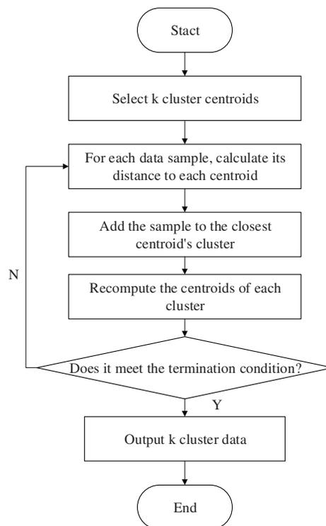
**Figure 3:** K-means clustering algorithm
