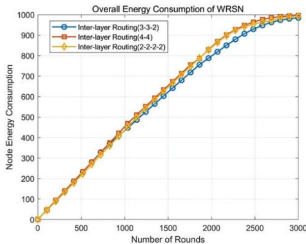
**Figure 12:** Trend of overall energy consumption in WRSN with three different inter-layer relay routing structures
