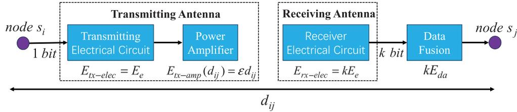
**Figure 1:** WRSN sensor node energy consumption model
