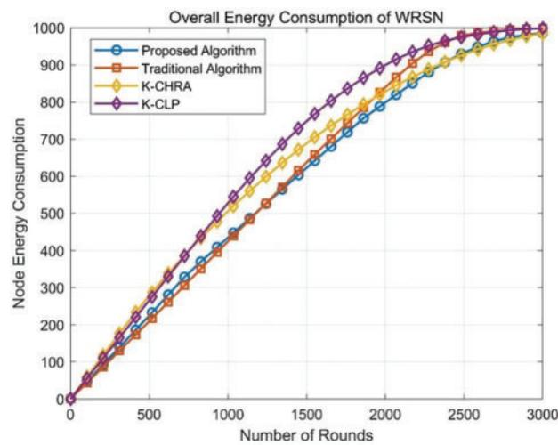
**Figure 15:** Structures trend of overall energy consumption for four algorithms in a 500-node WRSN
