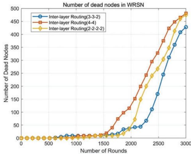
**Figure 11:** Trend of node death in WRSN with three different inter-layer relay routing structures
