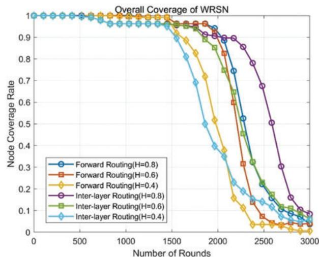
**Figure 10:** Trend of network coverage in WRSN with different thresholds under two routing mechanisms
