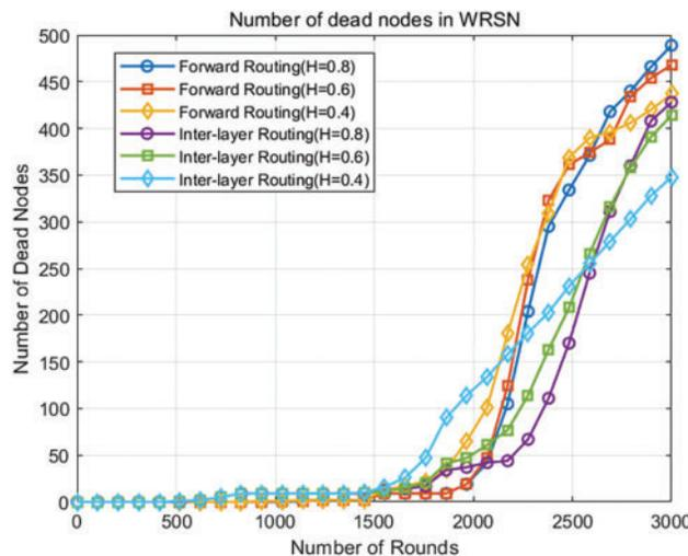
**Figure 8:** Trend of dead nodes in WRSN with different thresholds under two routing mechanisms
