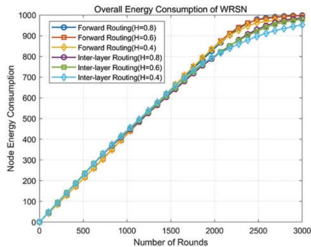
**Figure 9:** Trend of overall energy consumption in WRSN with different thresholds under two routing mechanisms
