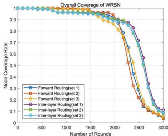
**Figure 7:** Trend of network coverage in WRSN under two routing mechanisms with different parameters
