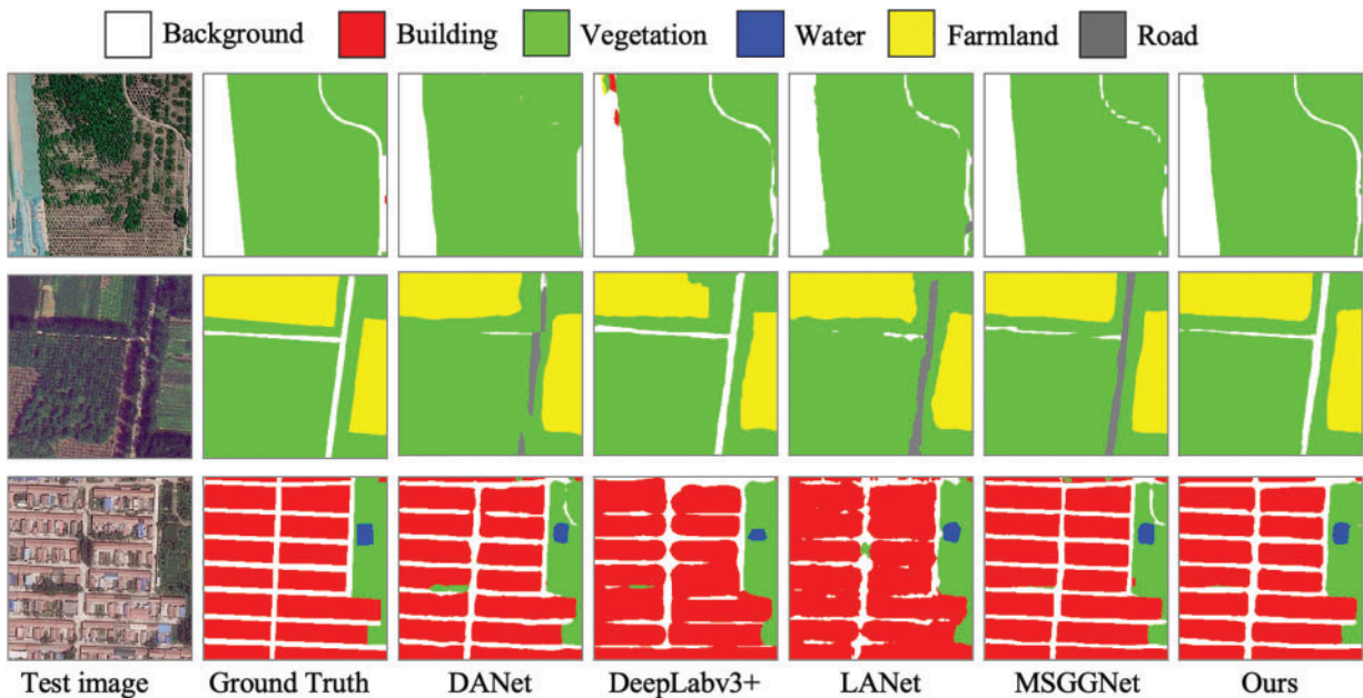
Figure 5: Visualization of segmentation outcomes for various methods applied to the BLU
