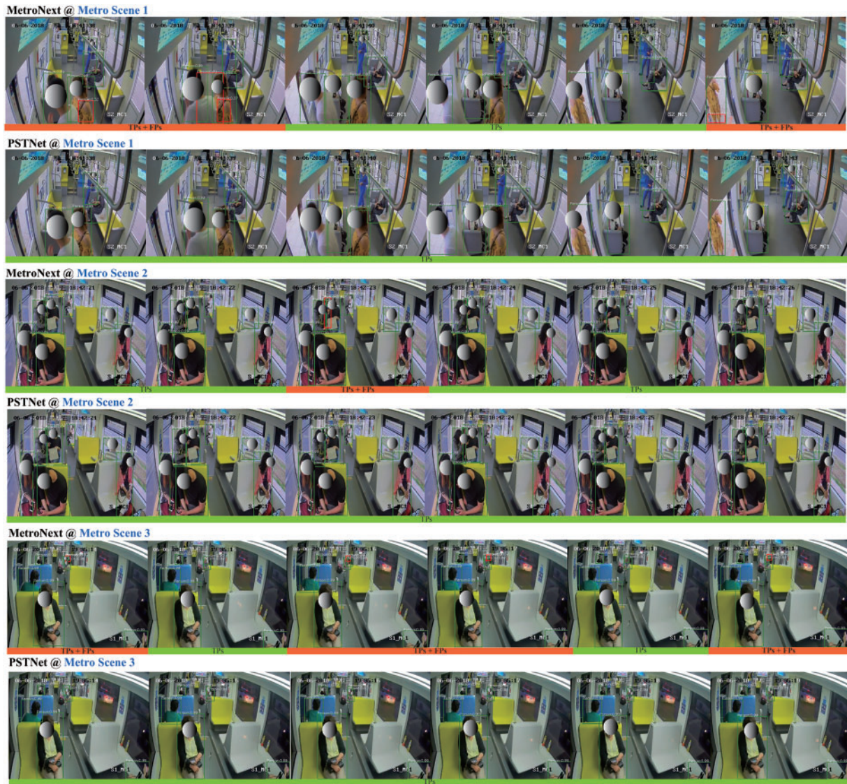
Figure 9: Comparing detection results of MetroNext and PSTNet on metro videos. “TPs” and “TPs+FPs” denote the True Positives and True Positives plus False Positives detection results, respectively. False Positives are drawn in red
