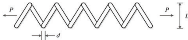
Figure 6: Schematic of the tension/compression spring design
