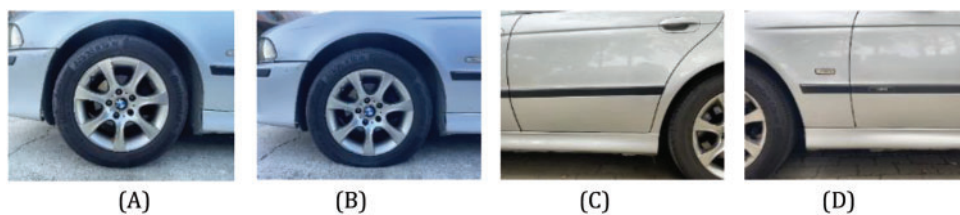
Figure 3: Pictures of car tires (A) Normal tire pressure; (B) Under-inflated tire; (C) and (D) No tire detected
