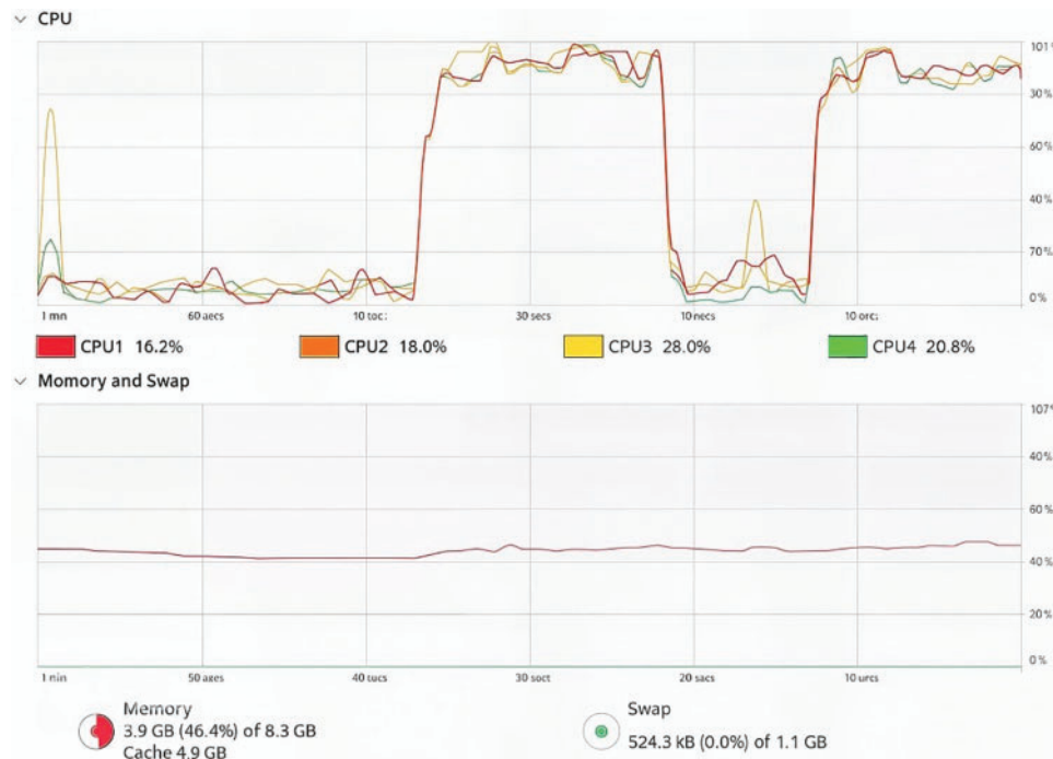
Figure 7: System resource usage during payload generation on Raspberry Pi 5
