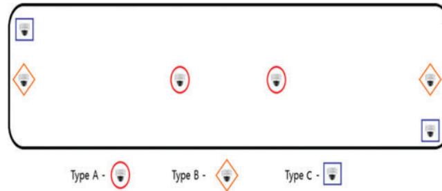
Figure 1: Layouts of CCTVs within railway vehicles
