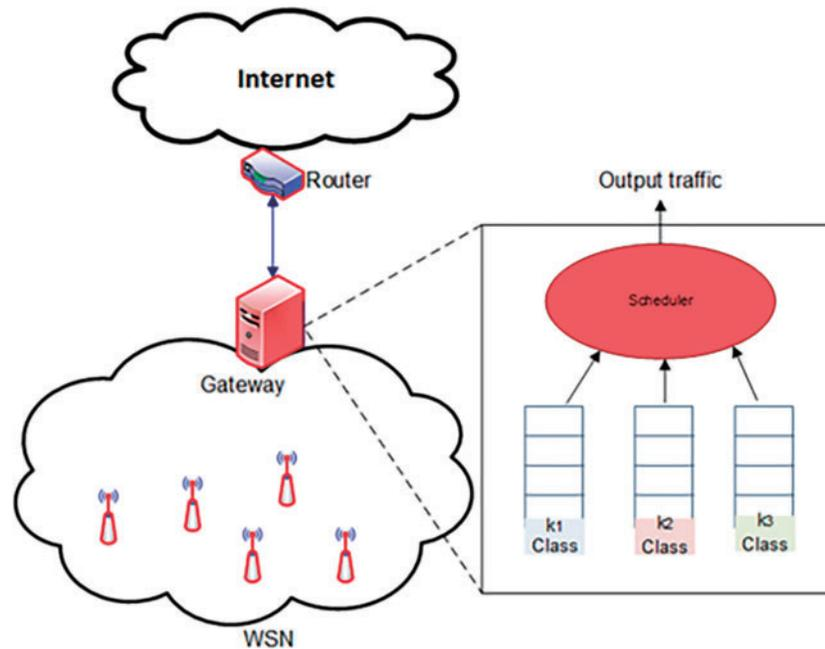
**Figure 1:** Traffic differentiation network model
