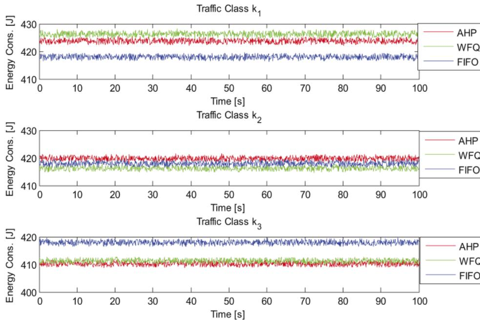
**Figure 8:** Energy consumption comparison for three scheduling algorithms (AHP, WFQ, FIFO)
