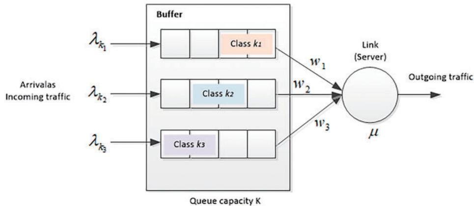
**Figure 2:** Queue system of the proposed model
