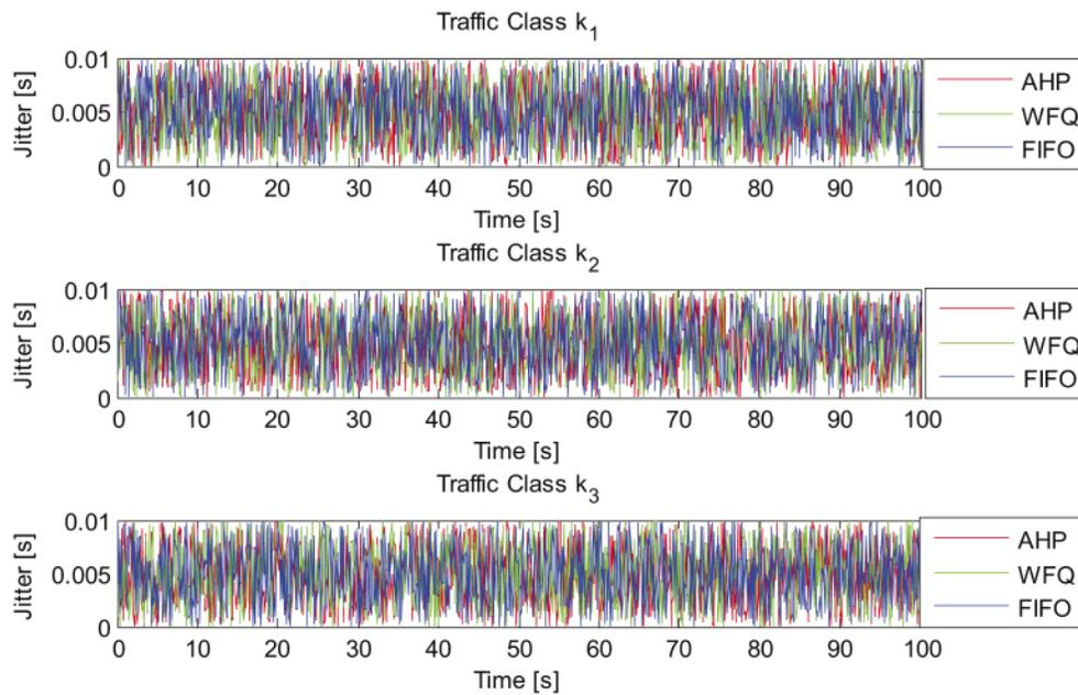
**Figure 7:** Jitter comparison for three scheduling algorithms (AHP, WFQ, FIFO) across traffic classes
