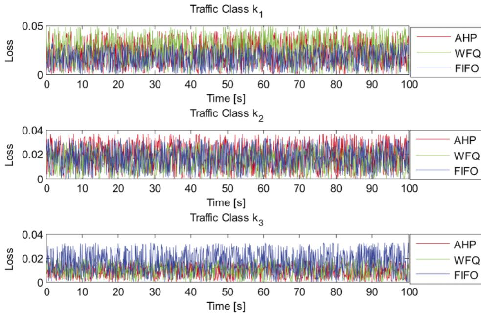
**Figure 6:** Packet loss comparison for three scheduling algorithms (AHP, WFQ, FIFO) across traffic class
