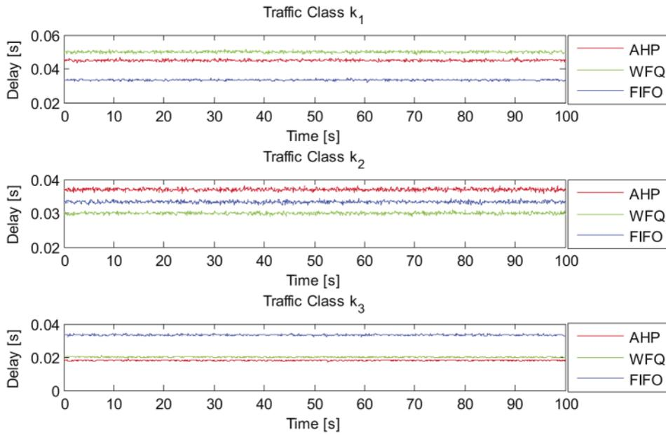
**Figure 5:** Delay comparison for three scheduling algorithms (AHP, WFQ, FIFO) across traffic classes
