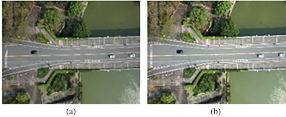
Figure 2: Contrast level enhancement using gamma correction (a) original images, (b) pre-processed images
