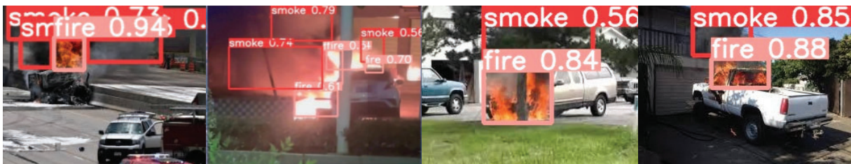
Figure 7: The detection results of smoke and fire
