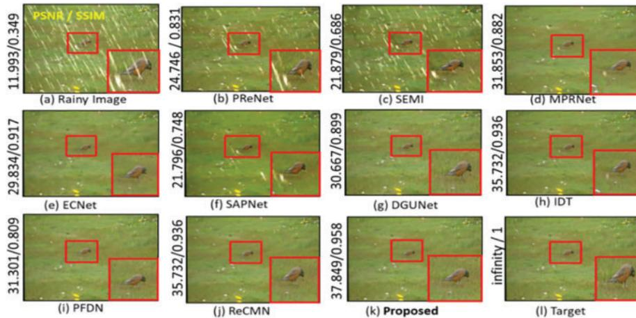
**Figure 4:** Visual results of existing SOTA networks and our network on Rain100L dataset
