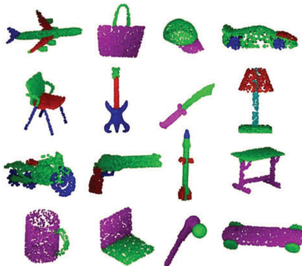
Figure 6: Part level semantic segmentation results on ShapeNet dataset. Semantic annotation using different colors for different parts
