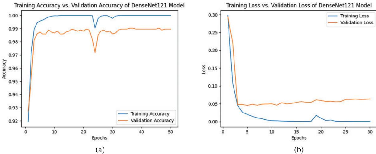
**Figure 10:** (a) Training and validation accuracy and (b) training and validation loss of DenseNet121
