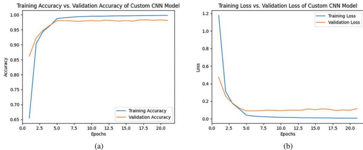
**Figure 5:** (a) Training and validation accuracy and (b) training and validation loss of custom CNN model
