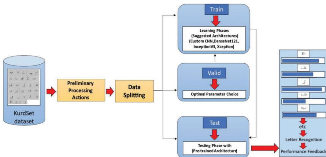
**Figure 4:** The flowchart of the proposed method for Arabic and Kurdish handwritten recognition
