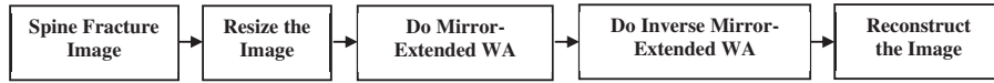
Figure 3: An algorithm for correcting the background of a spine fracture image using the inverse ME method
