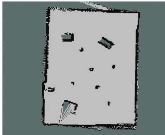
Figure 20: Mapping results of the traditional RRT autonomous exploration algorithm in actual environment 2
