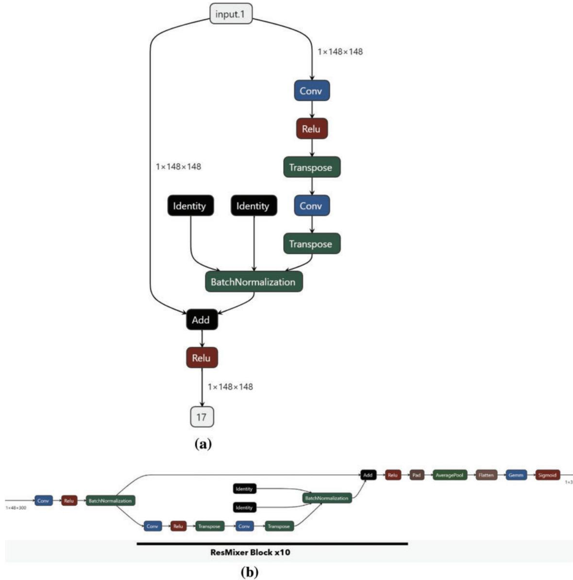
**Figure 8:** (a) Design of individual ResNet Mixer block. (b) The activity recognition network
