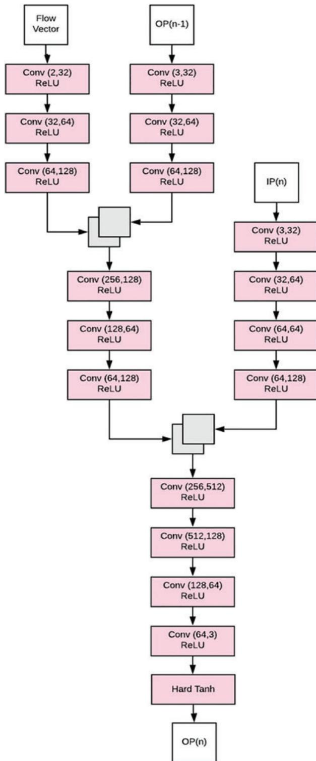
**Figure 3:** Video frame reconstruction network
