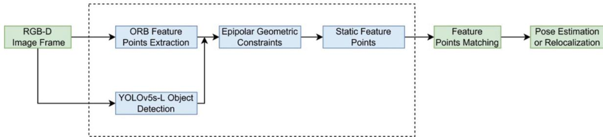
**Figure 8:** Visual odometer improved by YOLOv5s-L
