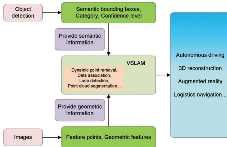
**Figure 6:** Visual SLAM framework based on object detection network
