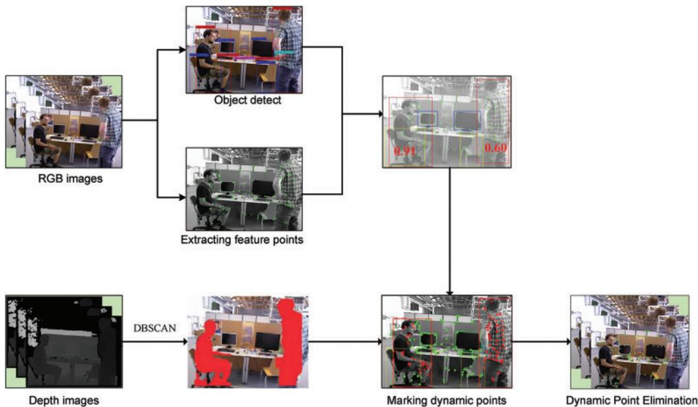
**Figure 9:** Dynamic point rejection method for CFP-SLAM. The image is from X. Hu’s paper “CFP-SLAM: A real-time visual SLAM based on coarse-to-fine probability in dynamic environments” [50]
