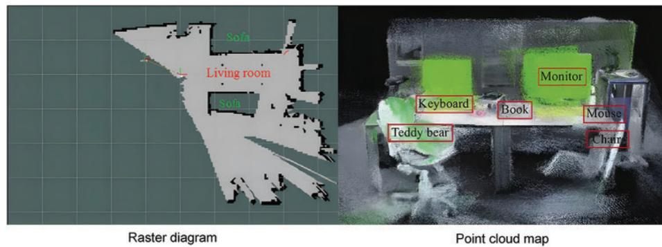
**Figure 14:** 2D raster map (left) and 3D point cloud map (right). The left image is from P. Maolanon’s paper “Indoor room identify and mapping with virtual-based SLAM using furniture and household objects relationship based on CNNs” [69]. The right image is from X. Hu’s paper “Semantic SLAM based on visual SLAM and object detection” [50]
