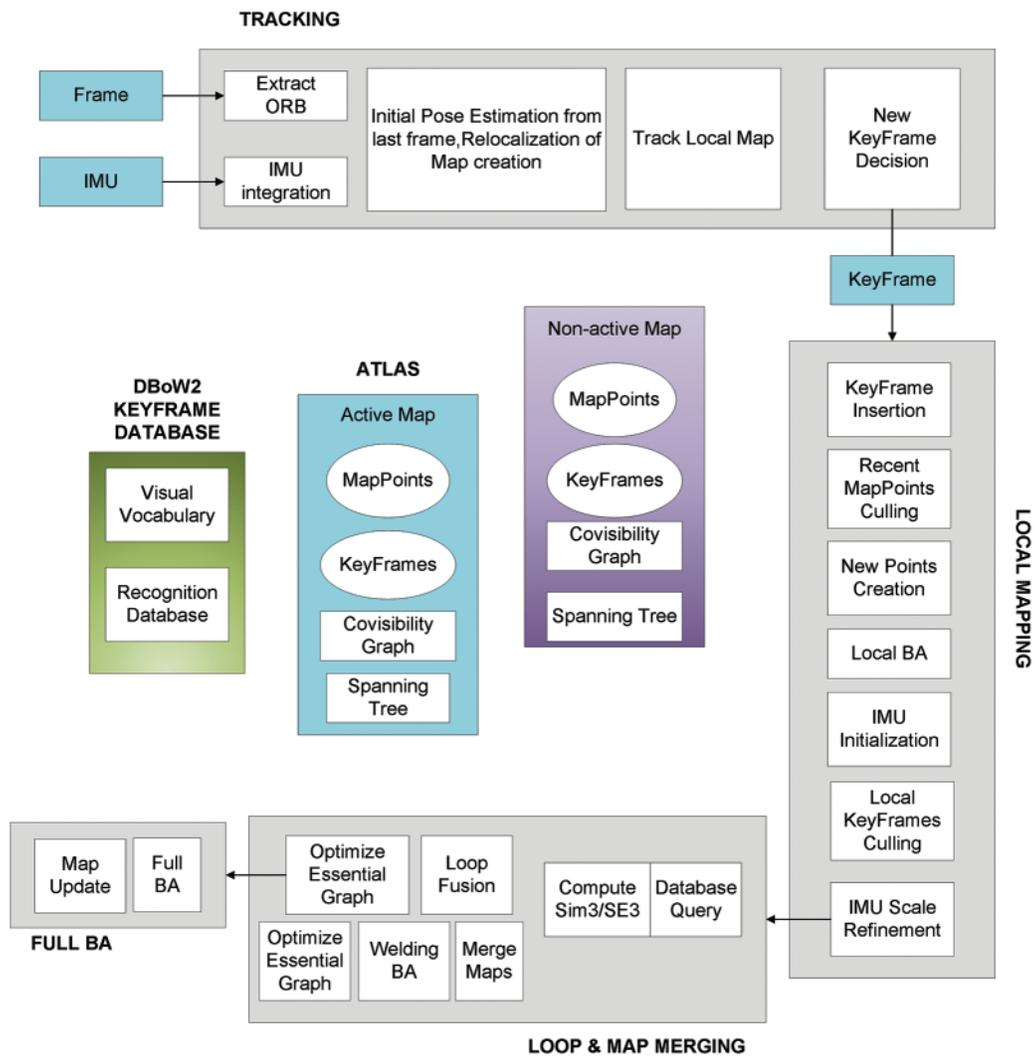
Figure 4: Main system components of ORB-SLAM3
