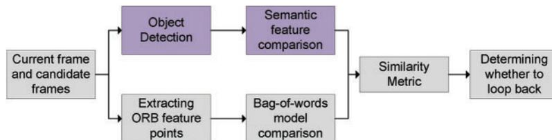
Figure 12: Loopback detection based on semantic bounding boxes
