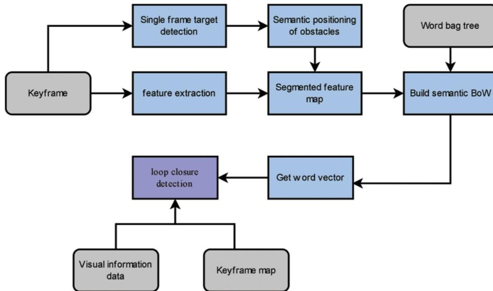
Figure 11: Semantic loop closure detection block diagram
