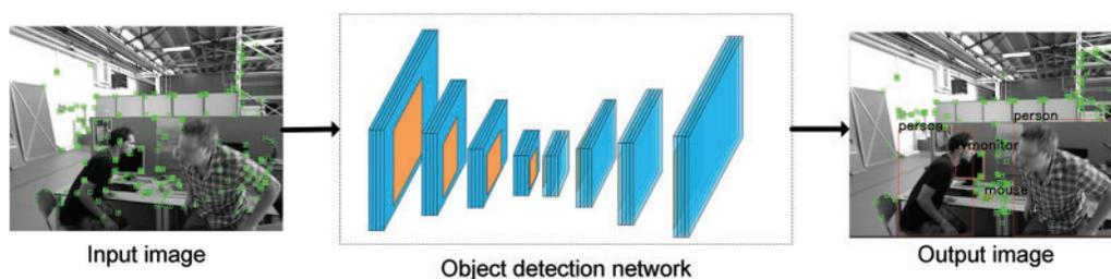
**Figure 7:** Eliminate dynamic points based on bounding box
