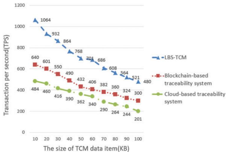
Figure 5: Comparison of TCM transaction processing capacity
