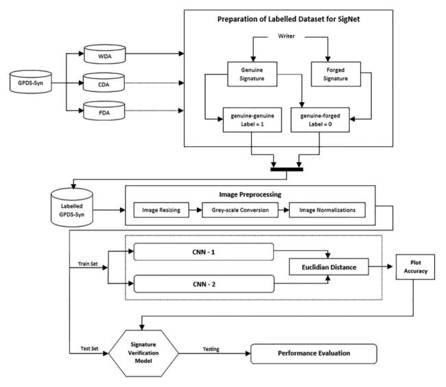
Figure 13: Block diagram of performance evaluation process on DL-based OfSV system
