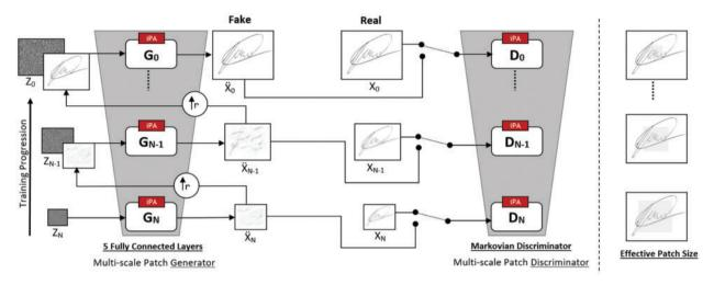
Figure 2: Architecture of OffSig-sinGAN, the proposed image augmentation model
