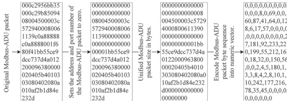
Figure 4: The whole process of data conversion
