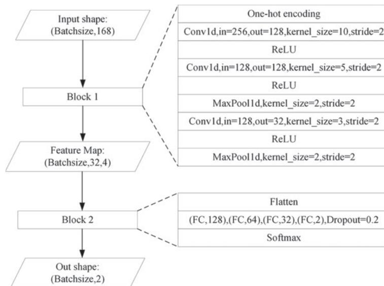
**Figure 7:** The parameter details of RRCNN
