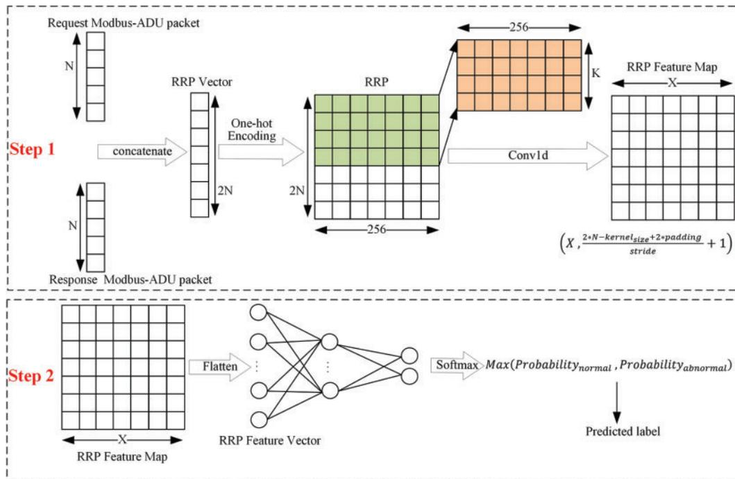
Figure 5: The overall structure of RRCNN
