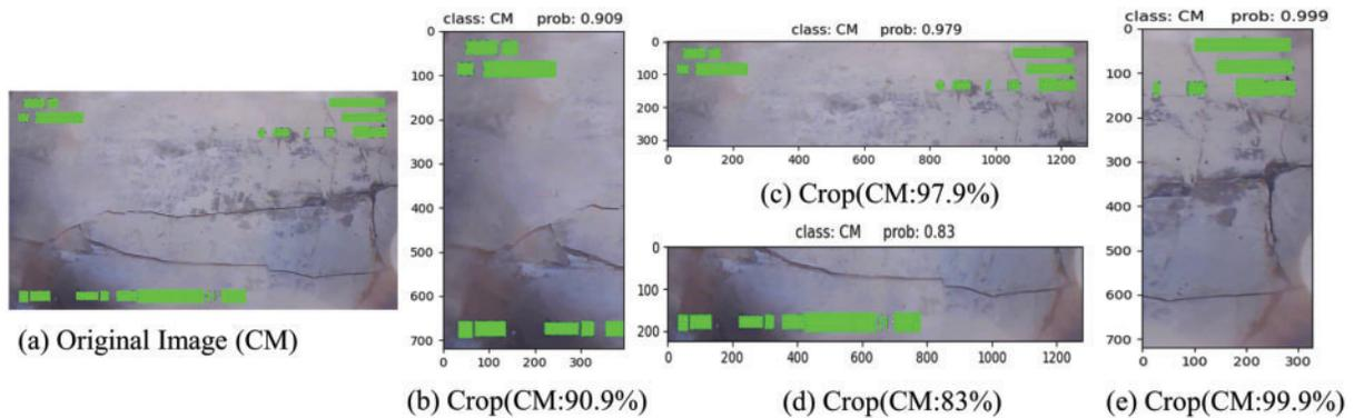
**Figure 9:** The prediction results of our proposed model on the cropped images. (a) represents the original image from the crack multiple class. (b–e) are the predicted results using our proposed model on randomly cropped images
