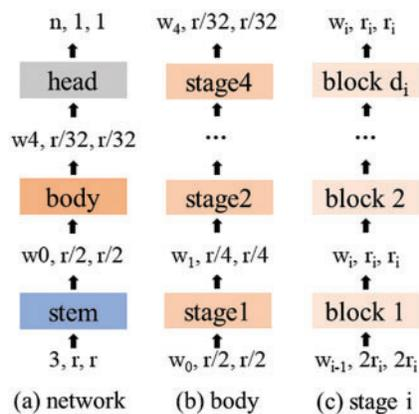
**Figure 3:** RegNet general network structures for deep learning models which consists of stem, body, and head part
