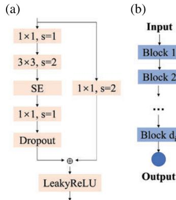
**Figure 6:** The block diagram of the proposed RegNet+ structure where s represents stride, SE represents sequence excitation block
