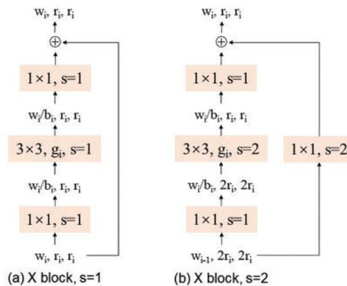
**Figure 4:** RegNet block structure based on the residual bottleneck block, where  $w$  represents the characteristic matrix's channel,  $g$  represents each group's group width, and  $b$  represents the bottleneck ratio
