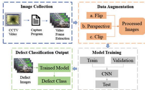
**Figure 1:** The comprehensive structure of the automated sewer condition monitoring system includes four major parts. (1) image collection from videos; (2) data augmentation on the acquired images; (3) CNN classification is used to train a different class of defects; (4) defect classification; and different models are trained to evaluate the performance of the proposed model with state of the models
