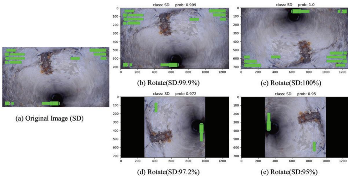
**Figure 10:** The prediction results of our proposed model on the rotated images. (a) represents the original image from the surface damage class. (b–e) are the predicted results using our proposed model on the rotated images
