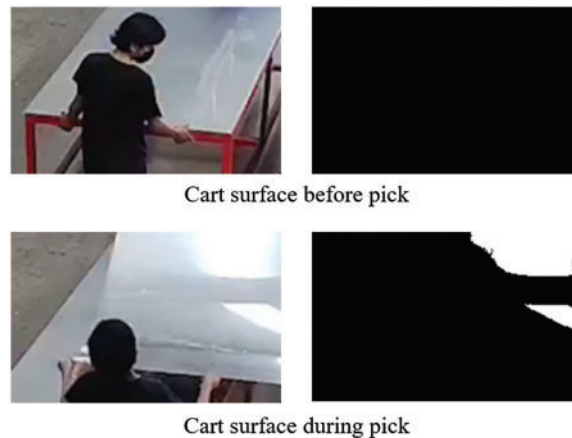
Figure 5: Pixels with their values within the defined range are activated and shown in white color
