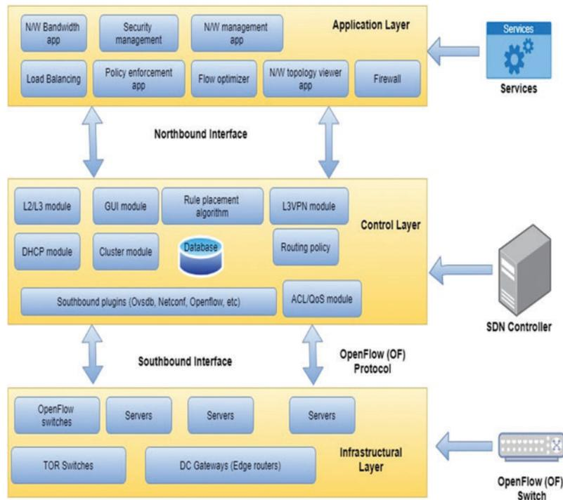
**Figure 2:** Three-layer SDN architecture
