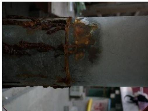
**Figure 2:** Rust overflows the surface of specimen
