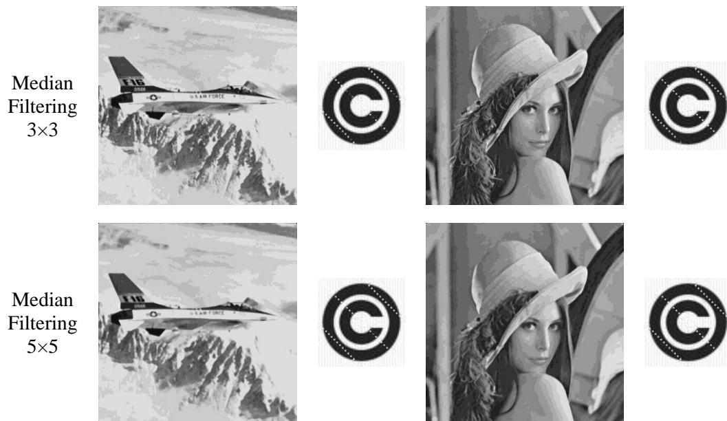
Figure 2: Average and Median Filtering Attacks with 3 \times 3 and 5 \times 5 filters and the extracted watermarks
