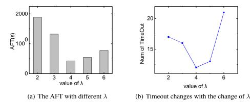
**Figure 4:** Performance evaluation with different  $\lambda$  when there are 30 concurrent flows with size of 300 KB
