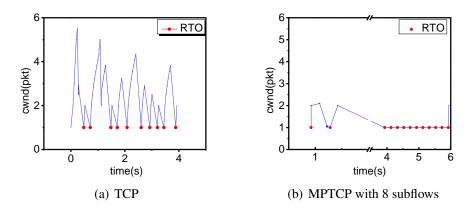
Figure 1: Evaluation of cwnd changes between TCP and MPTCP which contains 8 subflows
