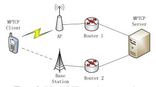
Figure 9: WLAN/LTE experiment scenario
