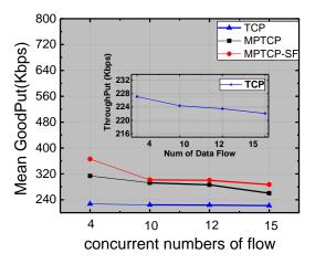
Figure 8: Throughput evaluation during long-flows transmission
