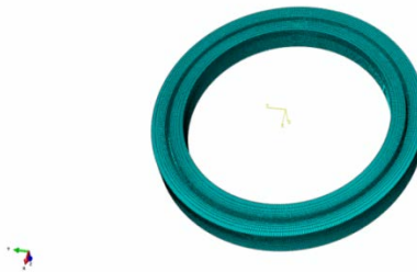
Figure 6: Finite element model of friction plate
