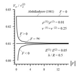
Figure 3: The dependence of the critical velocity on the imperfection parameter F in Case 1 (26) under h/R = 0.5
