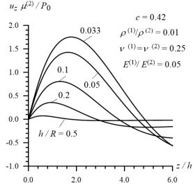
Figure 22: The distribution of the radial displacement  $u_z$  with respect to the coordinate z/h in Case 1
