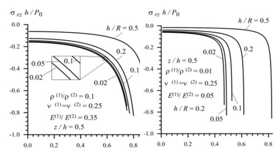
**Figure 12:** Dependence of the interface normal stress  $\sigma_{rz}$  on the dimensionless load moving velocity *c* in Case 1
