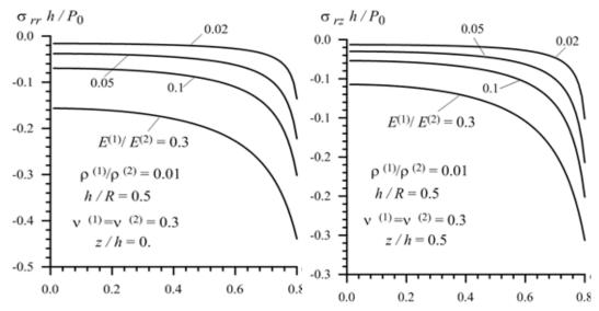
**Figure 14:** The influence of the modulus of elasticity of the cylinder material on the dependence between  $\sigma_{rr}$  and c in Case 1
