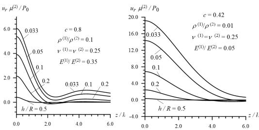
**Figure 20:** The distribution of the radial displacement  $u_r$  with respect to the coordinate z/h in Case 1
