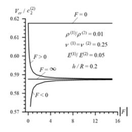
**Figure 6:** The dependence of the critical velocity on the imperfection parameter *F* in Case 1 (26) under h/R = 0.2
