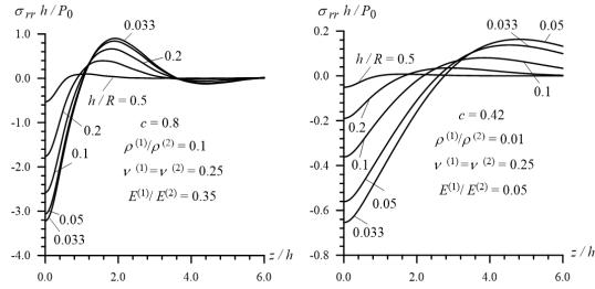
**Figure 16:** The distribution of the normal stress  $\sigma_{rr}$  with respect to the coordinate z/h in Case 1
