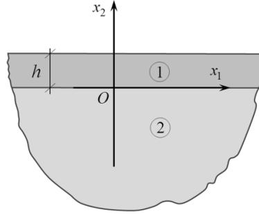
**Figure 1:** Geometry of the covered half-space.
