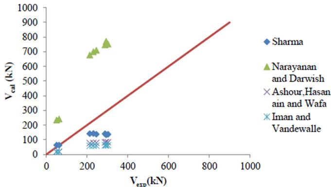
Figure 11: Comparison of calculated and experimental shear capacity.
