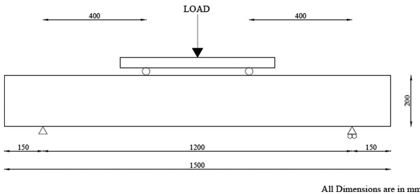
Figure 2: Two Point Loading Setup.
