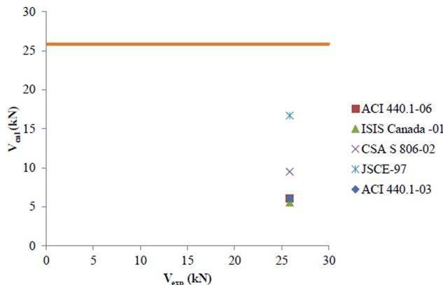
Figure 10: Comparison of calculated and experimental shear capacity for BFRP reinforced beams.
