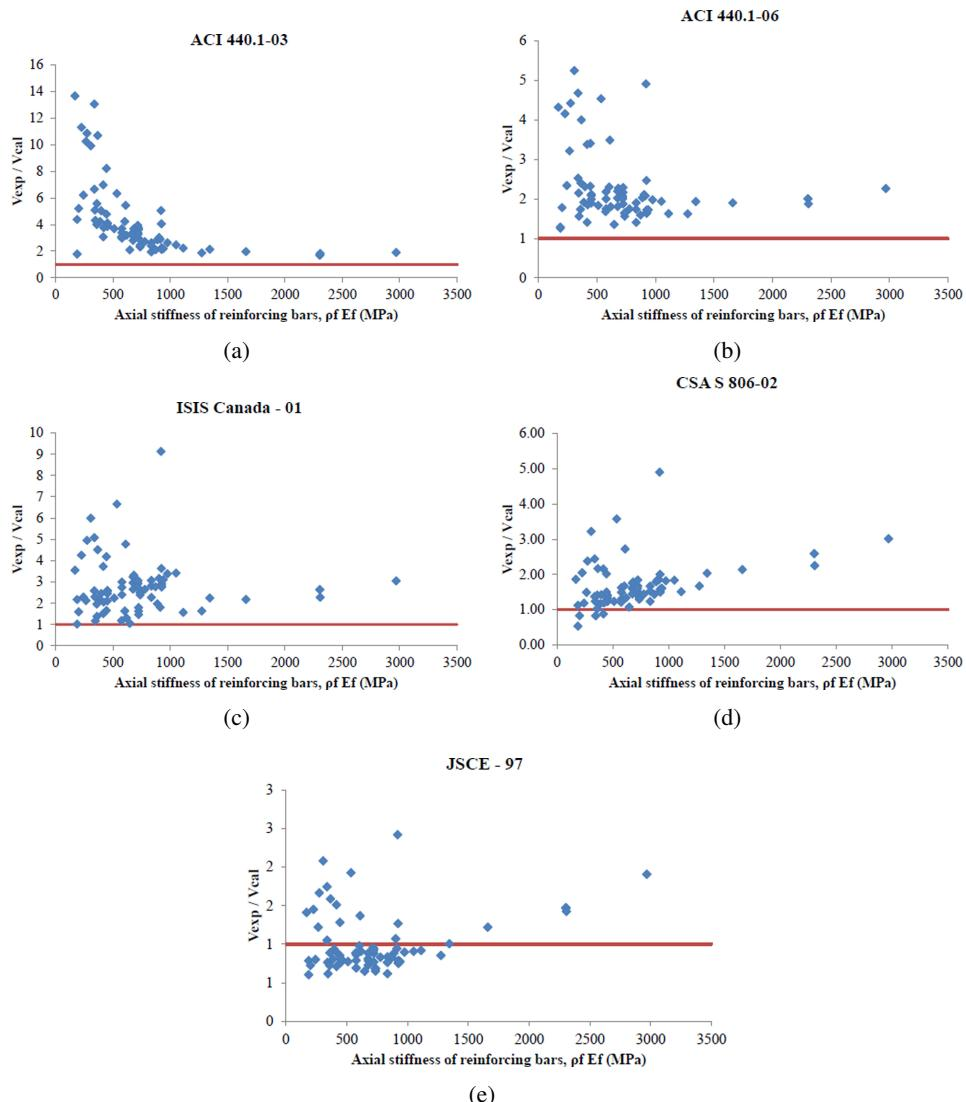
Figure 9: (a)–(e): Experimental to calculated shear strength versus Axial stiffness of reinforcing bars,  $\rho_f E_f$ .
