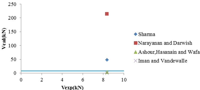
Figure 12: Comparison of calculated and experimental shear capacity for steel fiber reinforced beams.
