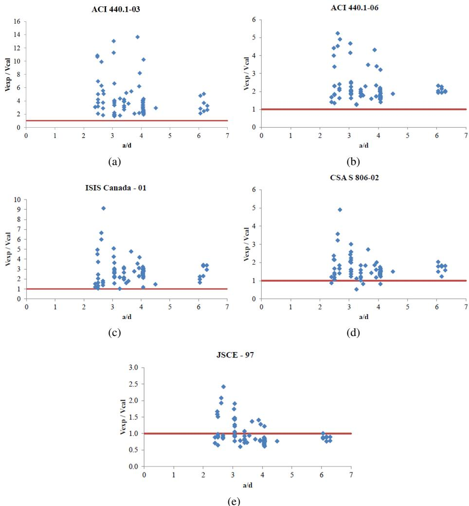
Figure 8: (a)–(e): Experimental to calculated shear strength versus shear span to depth ratio.
