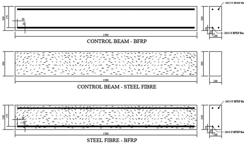
Figure 1: Description of Test Beam.
