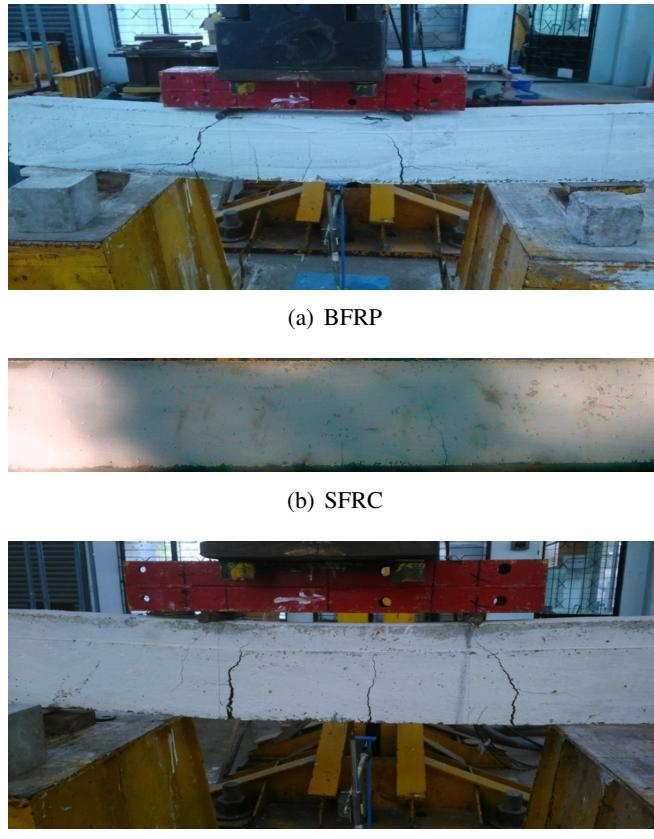
Figure 4: Failure patterns of beams.
