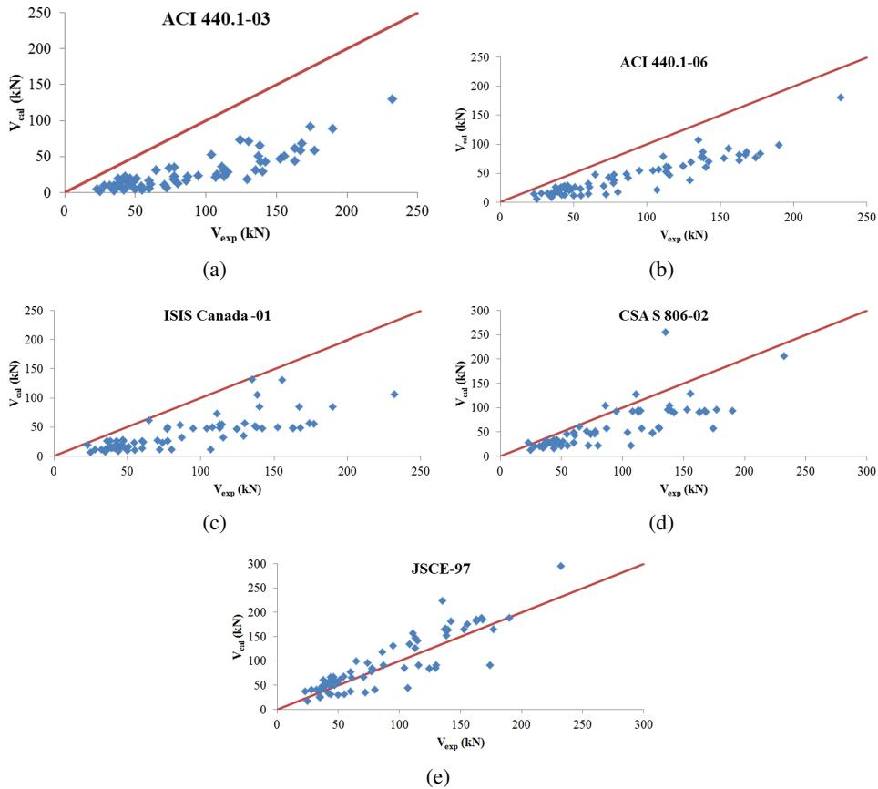
Figure 6: (a)–(e): Comparison of calculated and experimental shear capacity.
