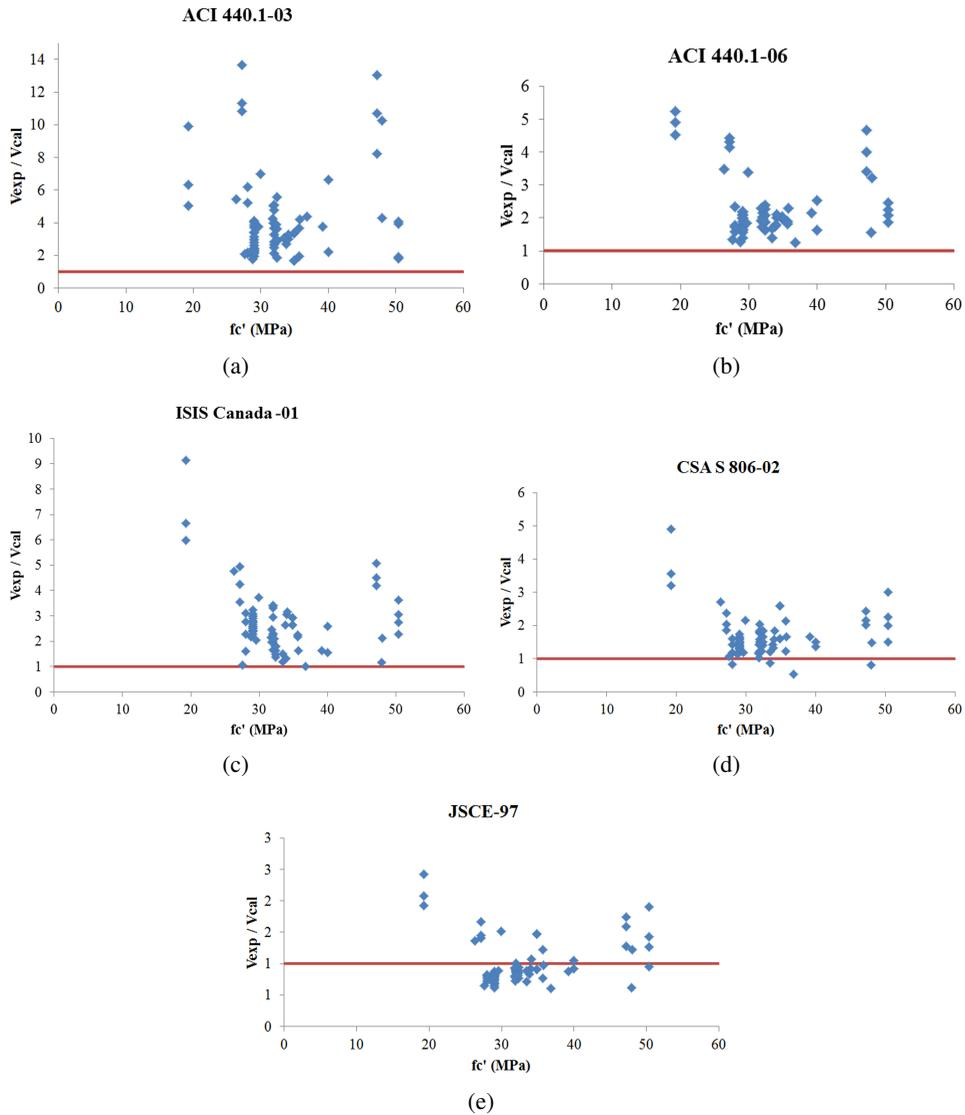
Figure 7: (a)–(e): Experimental to calculated shear strength versus concrete compressive strength.
