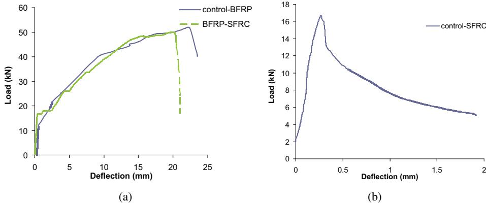
Figure 3: Load vs Deflection. (a) BFRP reinforced beams & SFRC-BFRP reinforced beam; (b) SFRC reinforced beams.
