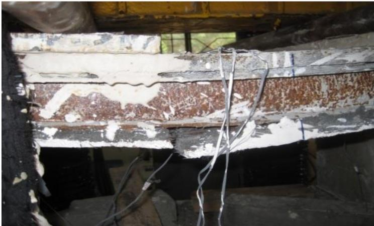
Figure 8(c): Failure of Bottom the midspan UHPC Panel.
