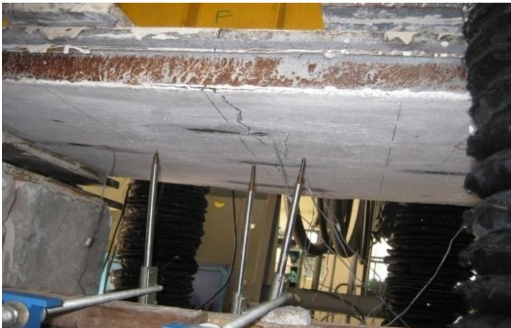
Figure 8(a): Initiation of the crack in the bottom UHPC.
