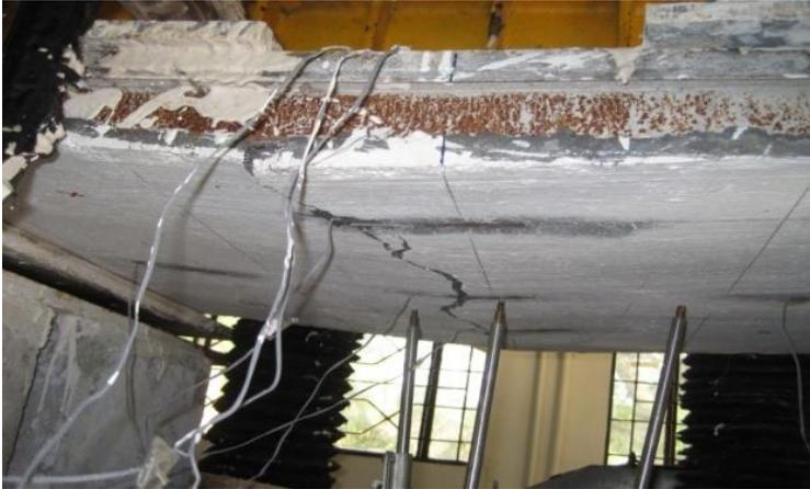
Figure 8(b): Growth of Crack along the midspan.
