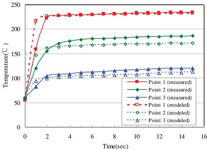
Figure 9: The modeled and measured temperature histories at the three reference points
