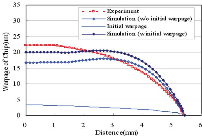
Figure 11: The modeled and measured warpage of the chip
