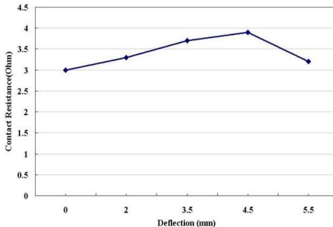
Figure 14: Measured contact electrical resistance versus deflection under FPB using four-point probe method
