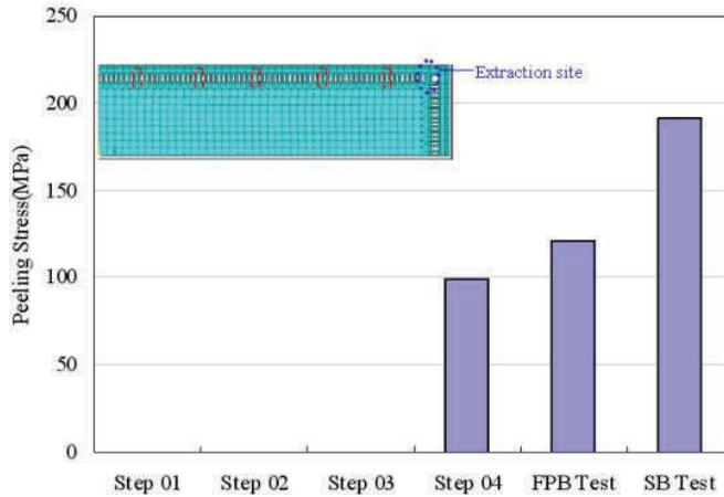
Figure 12: Peeling stresses of ACF versus 4 simulation steps and FPB and SB tests
