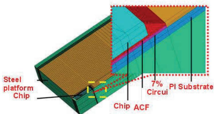
Figure 5: 3D thermal-mechanical FE model
