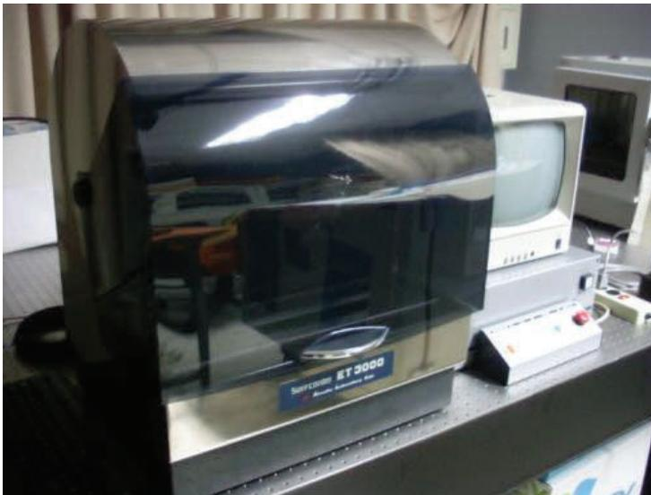
Figure 7: Micro figure Measuring Instrument (ET-3000)
