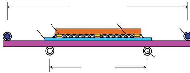
(a) Four point bending test (FPB)
