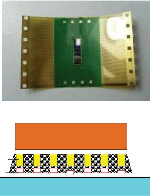
Figure 1: The TFCOF interconnect technology with ACF joints
