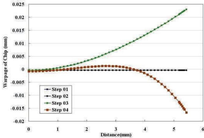
Figure 10: Process-induced warpage of the chip versus 4 simulation steps
