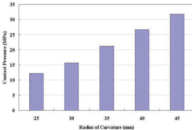
Figure 17: Modeled contact pressure versus bending curvature under SB
