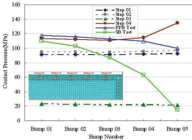
Figure 13: Contact stress of ACF joints versus 4 simulation steps and FPB and SB tests
