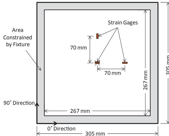
Figure 3: Strain Gage Locations on Instrumented Composite Panels
