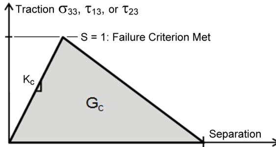
Figure 6: Cohesive Element Traction-Separation Relationship [Dassault Systèmes Simulia Corp (2011)]
