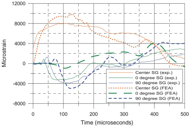
Figure 13: Strain Comparison, 24 ply Panel Impacted by 50.8 mm SHI at 116 m/s
