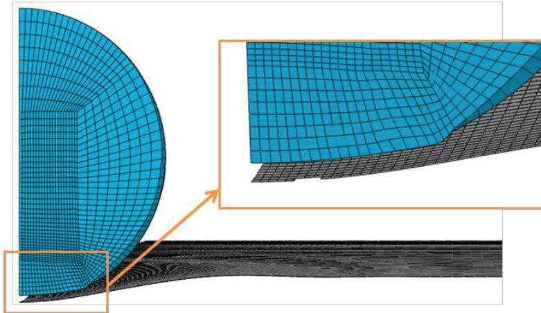
Figure 11: Elements Deleted From 6th Cohesive Element Layer (at Interface Between 6th and 7th Plies) Corresponding to Damage Initiation for 50.8 mm SHI Impact of 8 Ply Panel at 70 m/s
