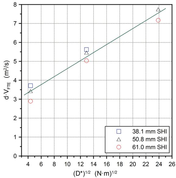
Figure 17: SHI Diameter Times Critical Velocity Versus Effective Bending Stiffness
