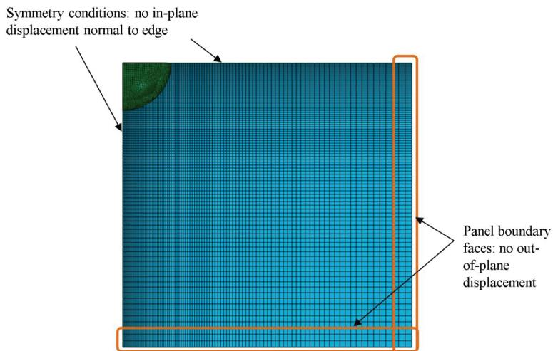
Figure 5: Top View of Panel and SHI Impact, Showing Symmetry Planes and Boundary Condition Areas
