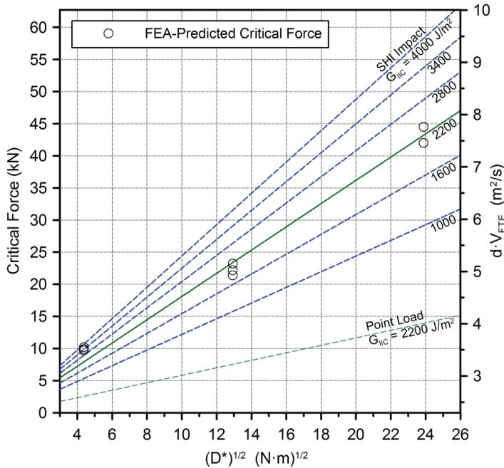
Figure 18: Scaling of Critical Force with Interlaminar Properties and Effective Bending Stiffness; Mapping Between Vertical Axes via  $(dV_{FTE} = 0.123F_{crit} + 2.29)$  (Linear Fit,  $R^2 = 0.95$ )
