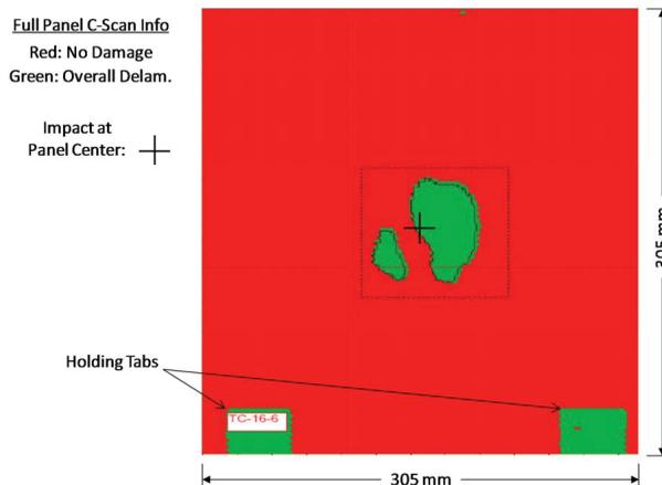
Figure 15: Delamination Shape Near FTE for 16 Ply Panel Impacted With 38.1 mm SHI at 162 m/s; Green Color Indicates Overall Delamination Existing at Any Plane Within the Laminate, Red Color Indicates No Delamination
