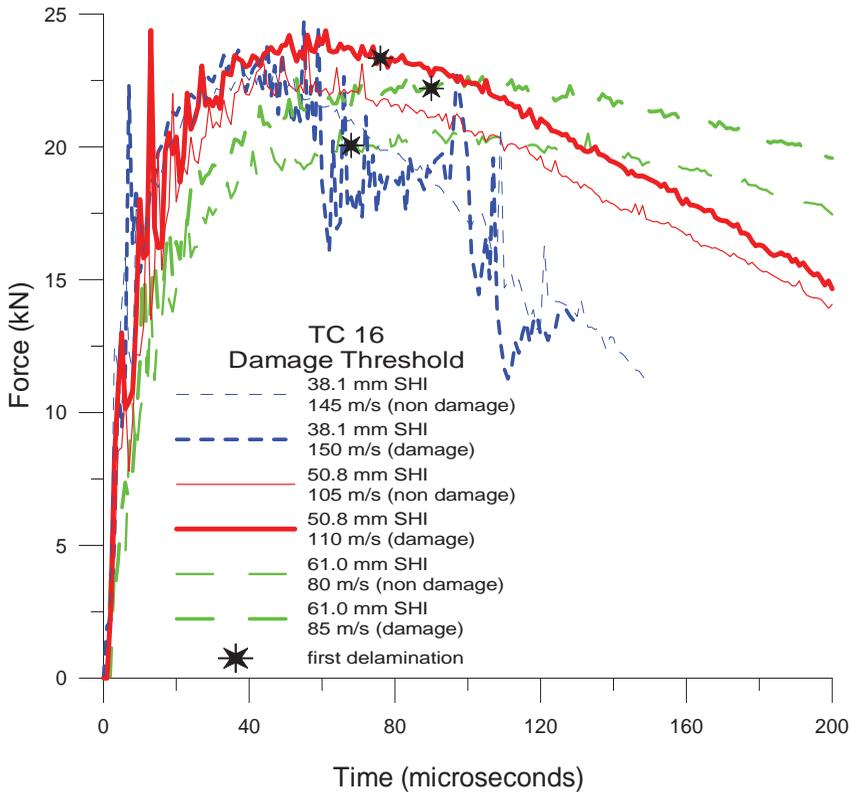
Figure 9: Force Histories for the Bounding Velocities of 16 Ply Panels
