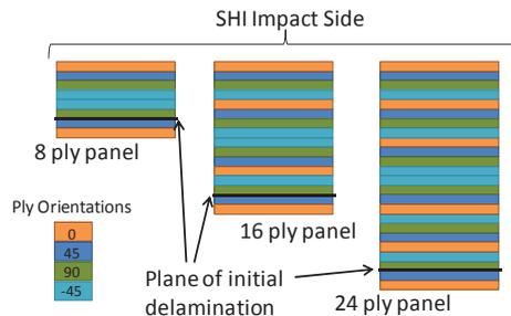
Figure 14: FEA Damage Initiation Plane in Panels
