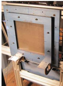
(c) Composite Panel in Picture Frame Fixture (12.7 mm Steel with 267x267 mm Opening)
