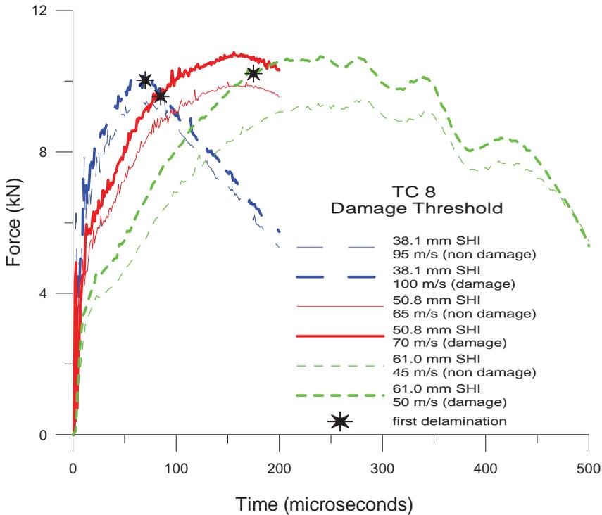
Figure 8: Force Histories for the Bounding Velocities of 8 Ply Panels
