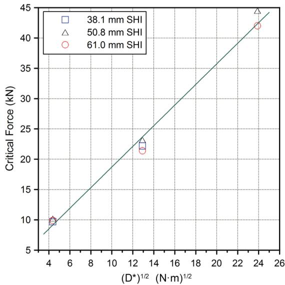
Figure 16: Critical Force Versus Effective Bending Stiffness
