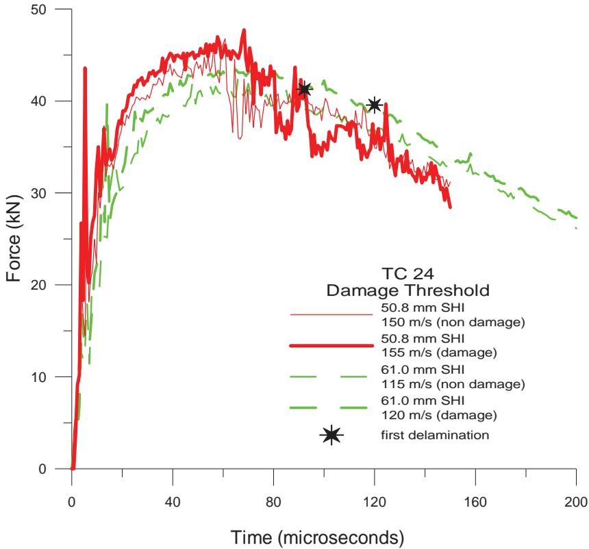
Figure 10: Force Histories for the Bounding Velocities of 24 Ply Panels
