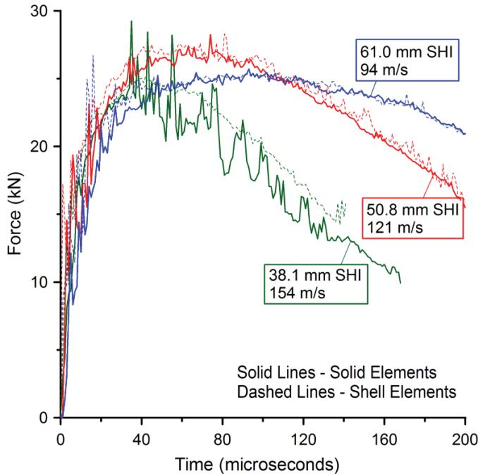
Figure 19: Comparison of Force Histories for Shell Element and Solid Element Models of 16 Ply Panels
