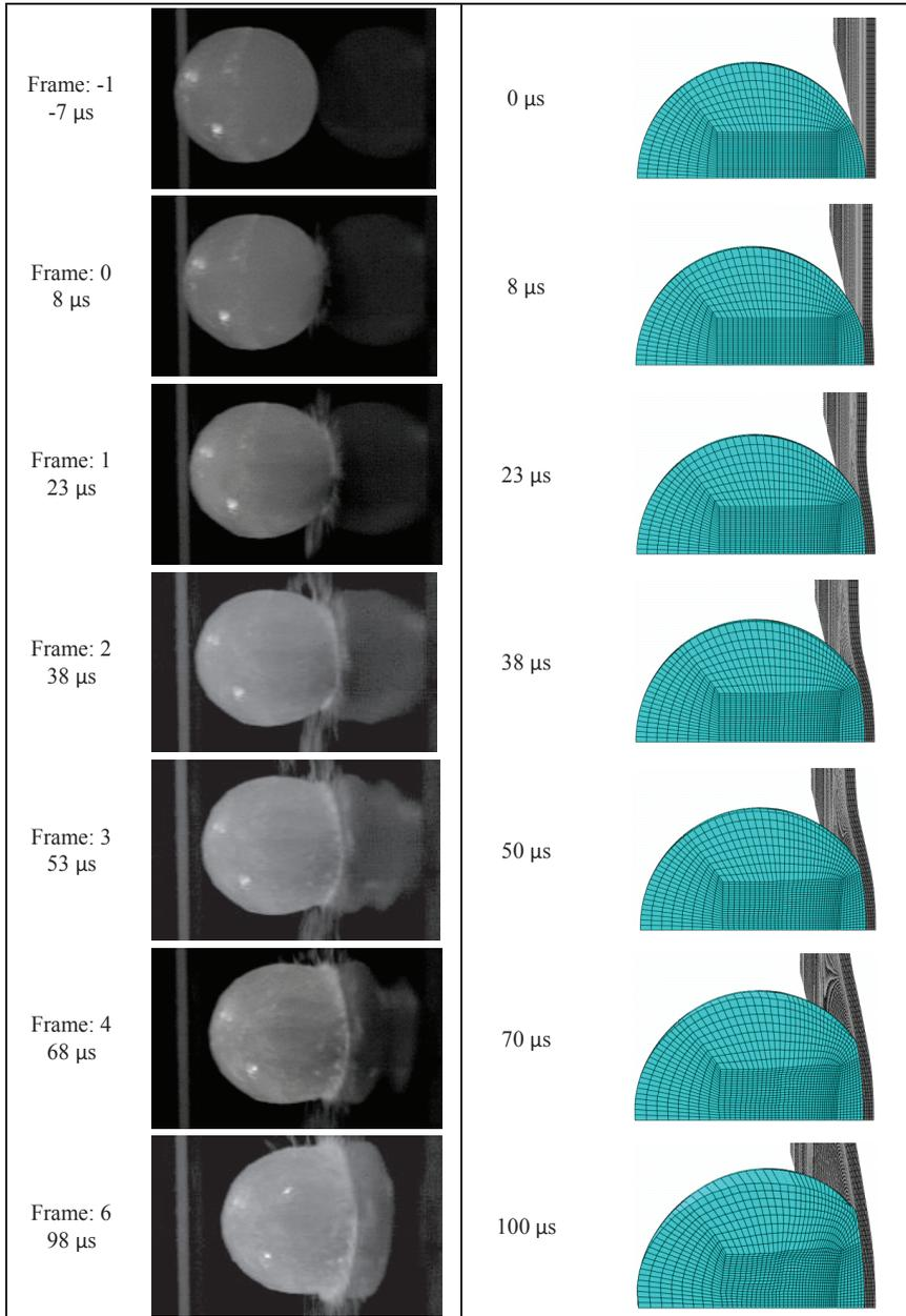
Figure 7: Comparison of Predicted and Experimentally-Observed Deformations of 38.1 mm SHI Impacting 8 Ply Panel at 126 m/s
