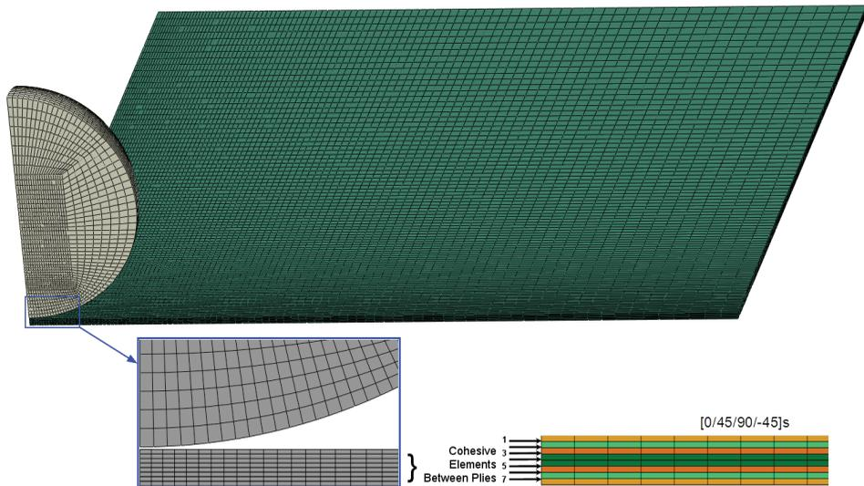
Figure 4: Quarter-Symmetric Mesh for Ply Panel and 50.8 mm SHI; Cohesive Element Details
