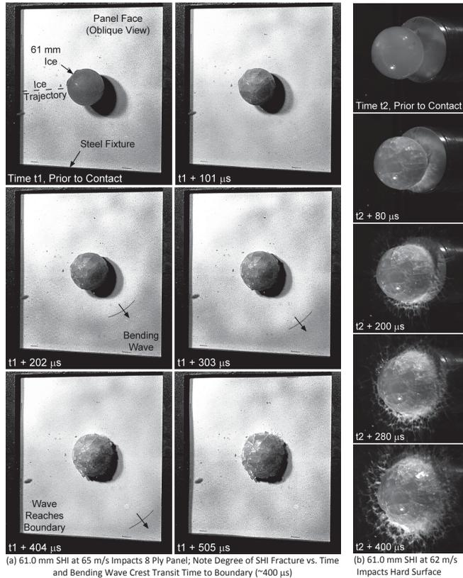
Figure 2: High Speed Video Still Images Comparing Degree of Crushing of 61.0 mm SHI Impacting (a) 8 Ply Panel and (b) Nearly Rigid Hard Surface; Times  $t_1 < 101\mu s$  and  $t_2 < 40\mu s$  Show One Video Frame Just Prior to Contact
