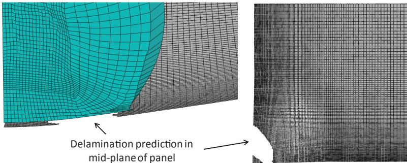
Figure 12: Elements Deleted From 4th Cohesive Element Layer (at Interface Between 4th and 5th Plies) Showing Extent of Delamination Resulting from 50.8 mm SHI Impact of 8 Ply Panel at 95 m/s (1.35xFTV)
