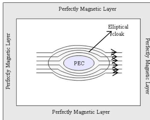
Figure 3: Full-wave simulations domain of elliptical-cylindrical cloaks. The cloaking object is an elliptical cylindrical PEC, and the cloak was made up of anisotropic material.
