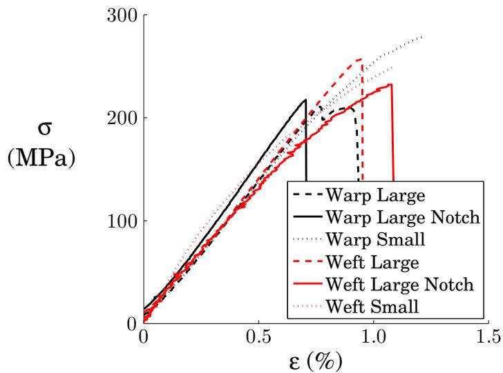
Figure 10: Static compression test results for 6% Z-fiber reinforced composite material Pankow, Salvi, Waas, Yen, and Ghiorse (2011).
