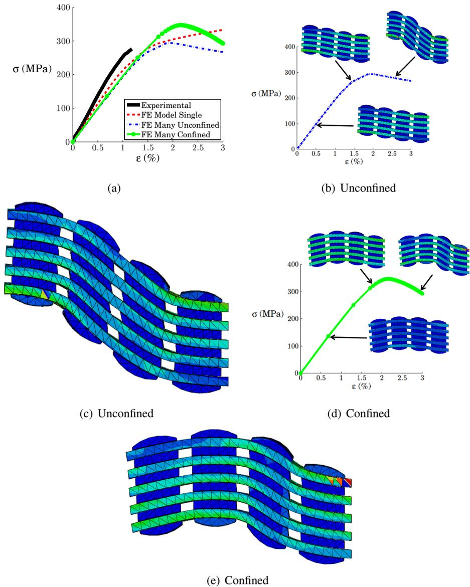
Figure 19: Macroscopic stress vs. macroscopic strain response comparison of static results comparing the different models. Von Mises strain contours are shown.
