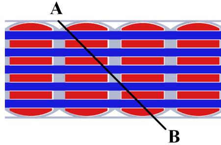
Figure 16: Required path for proper kink band formation in RUC model. Note that it will travel across multiple Z-fibers during formation
