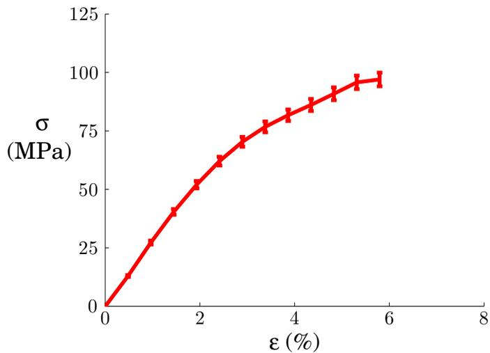
Figure 3: Quasi-static stress vs. strain curve for SC-15 matrix material.
