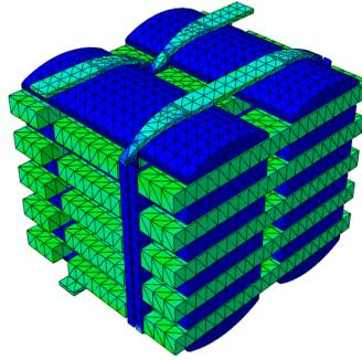
Figure 12: RVE of 3D woven geometry. The matrix material has been removed showing only the fiber tow bundles.
