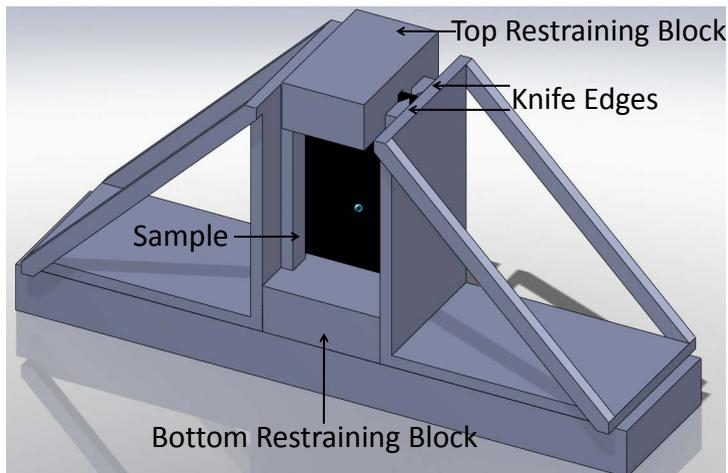
Figure 8: Large Compression fixture with anti-buckling guides.
