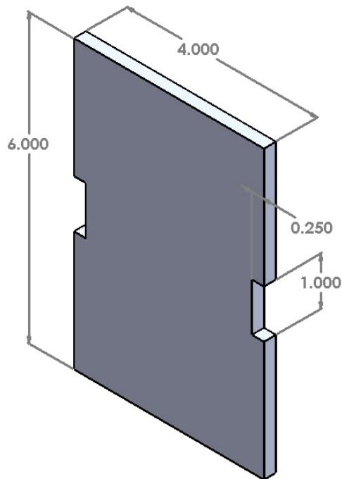
Figure 9: Large compression sample with notch shown to promote failure in the gauge section.
