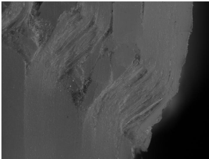
Figure 7: Microscopic images of kink bands obtained in the quasi-static compression tests Pankow, Salvi, Waas, Yen, and Ghiorse (2011).
