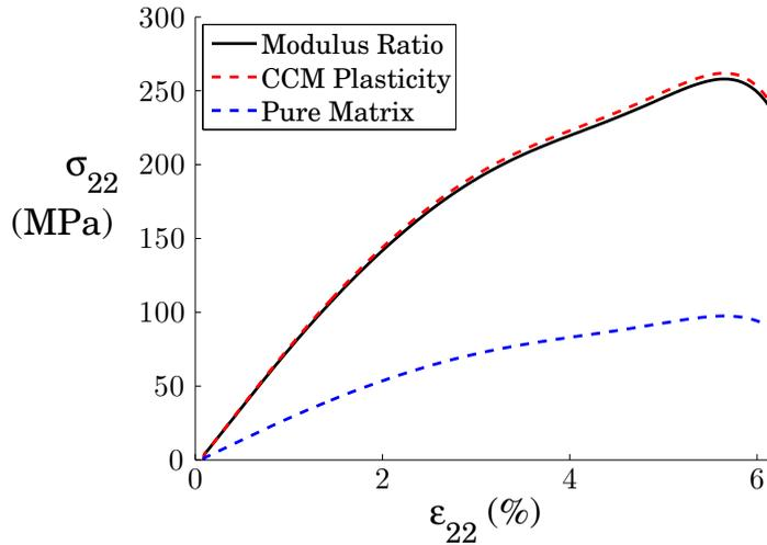
Figure 4: Comparison of the two different methods for calculating the stress vs. strain response of a fiber tow bundle in the transverse direction.
