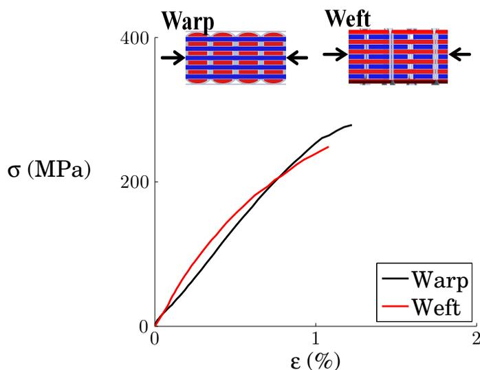
Figure 5: Quasi-static compression response of 6% Z-fiber reinforced composite Pankow, Salvi, Waas, Yen, and Ghiorse (2011).
