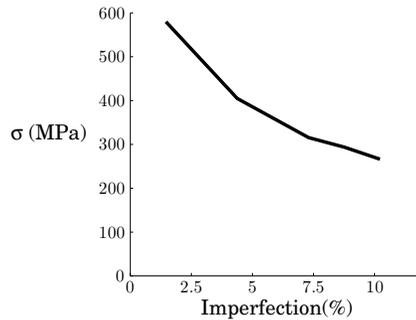
Figure 18: Comparison of imperfection to max strength for unconfined specimen.
