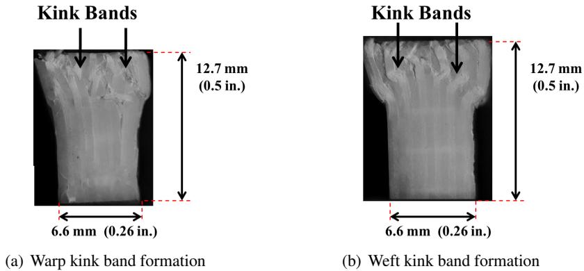
Figure 6: Comparison of the quasi-static failure modes in the composite material. Pankow, Salvi, Waas, Yen, and Ghiorse (2011)
