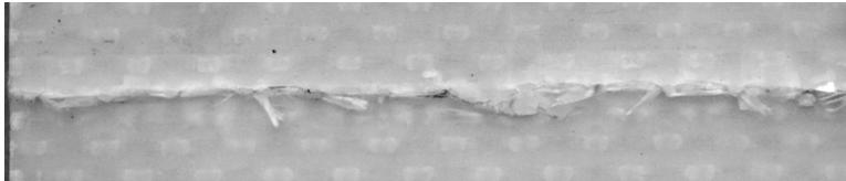
(b) Perpendicular surface to the kink band formation showing a single kink band that forms all the way across the specimen.
