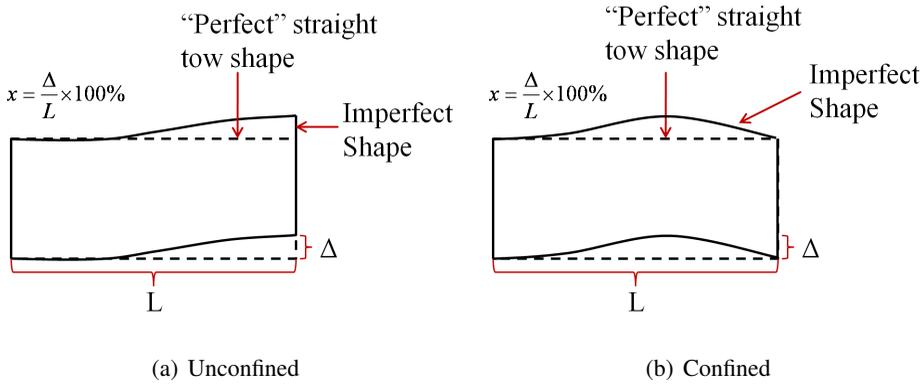
Figure 17: Amplitude perturbation to seed initial imperfection.
