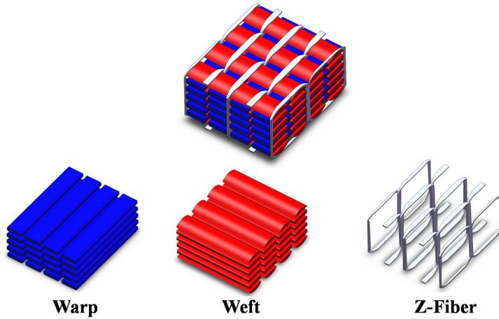
Figure 1: Representative Geometry of 3D woven RUC geometry.
