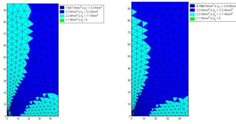
Figure 18: Axial stress analysis on the longitudinal section for plain concrete
