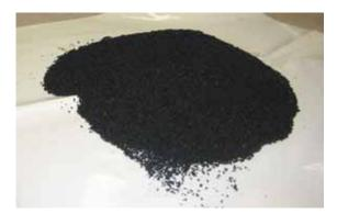
Figure 28: Gommamica Powerfill ECO (SBR Styrene Butadiene Rubber) rubber coarse aggregate, commercialized by Elastrade Srl
