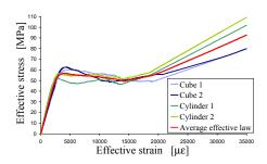
Figure 40: Effective stress-effective strain diagrams for cubic and cylindrical specimens and average effective law for Mixture 1
