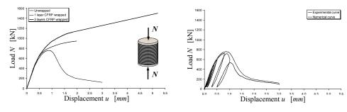
Figure 20: Numerical loaddisplacement curves for unwrapped and CFRP wrapped specimens
