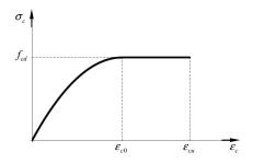
Figure 44: Design stress-strain diagram for concrete
