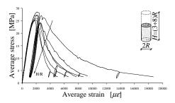
Figure 10: Size effect for the average stress-average strain diagrams
