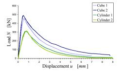
Figure 41: Load-displacement diagrams for Mixture 2
