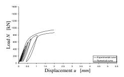
Figure 22: Numerical and experimental results for the one-layer CFRP wrapped specimens
