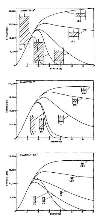
Figure 24: Influence of specimen shape on the  $\bar{\sigma} - \bar{\epsilon}$  curve for marble loaded in uniaxial compression [Hudson Brown and Fairhurst (1971)]
