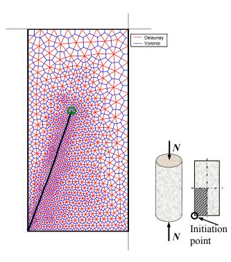
Figure 16: Crack path for the bottom-left quarter of the longitudinal section
