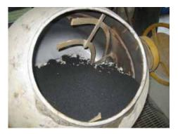
Figure 29: Laboratory batch mixer
