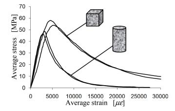
Figure 27: Shape-effect for cubic and cylindrical concrete specimens
