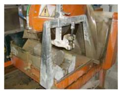
Figure 32: Automatic cylinder-end grinder
