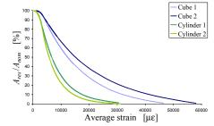
Figure 42: Shape-effect on the decrement of resistant area for Mixture 2
