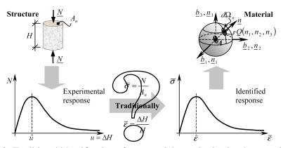
Figure 3: Traditional identification of mono-axial constitutive law by experimental tests
