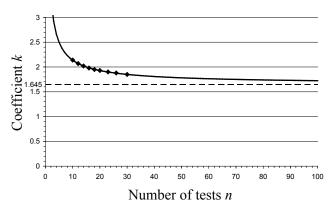
Figure 45: Interpolation of the coefficient *k* (90% confidence degree)
