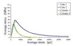
Figure 38: Shape-effect on the average stress-average strain diagrams for Mixture 1
