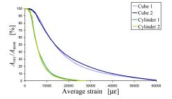
Figure 39: Shape-effect on the decrement of resistant area for Mixture 1
