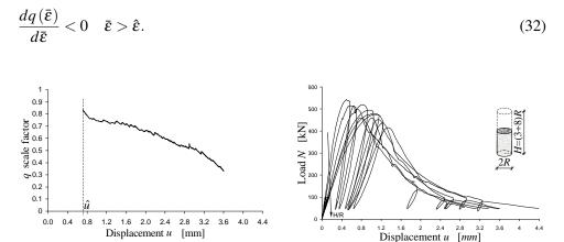
Figure 8: Scale factor between the percentage resistant area and normalized load laws
