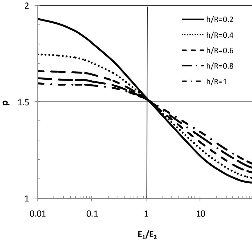
Figure 9: Variation of the power coefficient,  $p$ , as a function of film modulus ( $E_1/E_2$ ).
