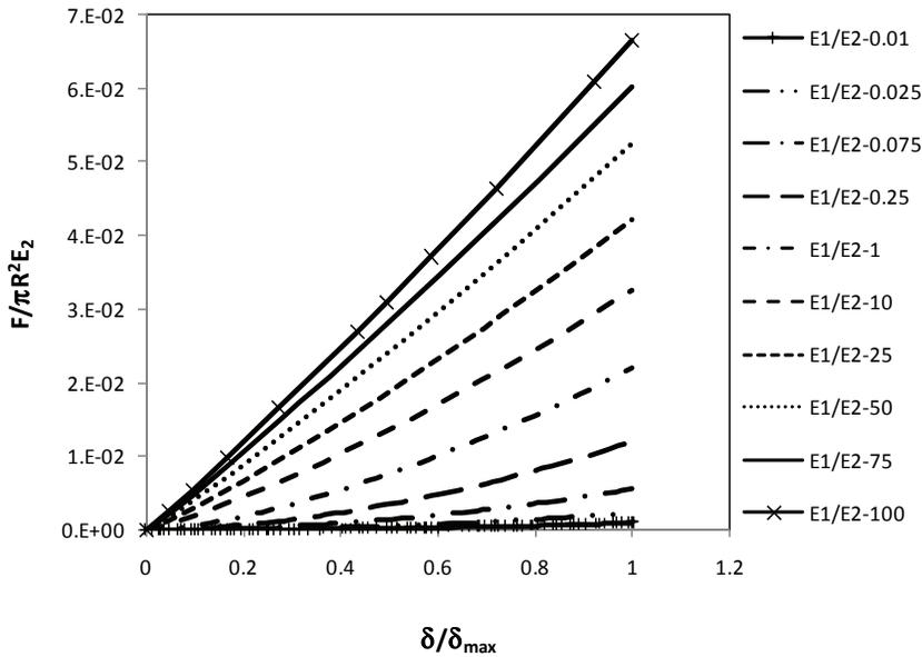
Figure 4: typical indentation load-displacement curves for the film-substrate structures. The film thickness  $h/R=0.2$ .
