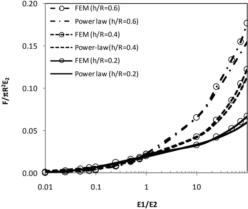
Figure 7: Comparisons of the FEM results and the generalized power law predictions: maximum indentation force vs. film modulus.
