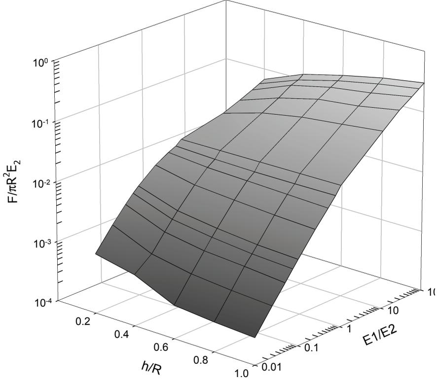
Figure 5: Maximum indentation load as functions of normalized film modulus ( $E_1/E_2$ ) and normalized film thickness ( $h/R$ ). The film Poisson's ratio is  $E_1/E_2=1$ .
