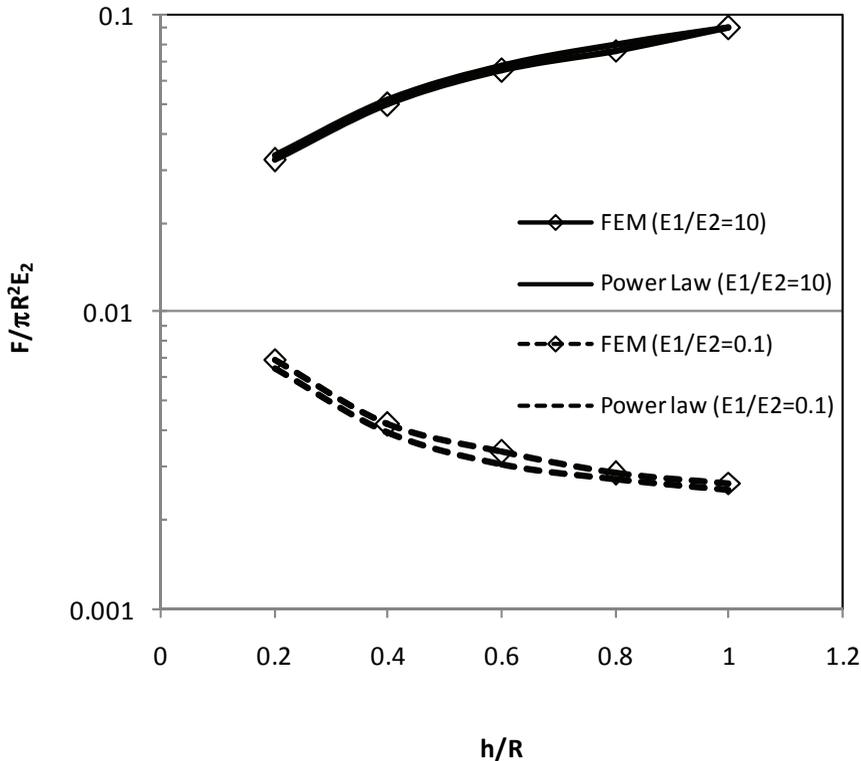
Figure 8: Comparisons of the FEM results and the generalized power law predictions: maximum indentation force vs. film thickness.
