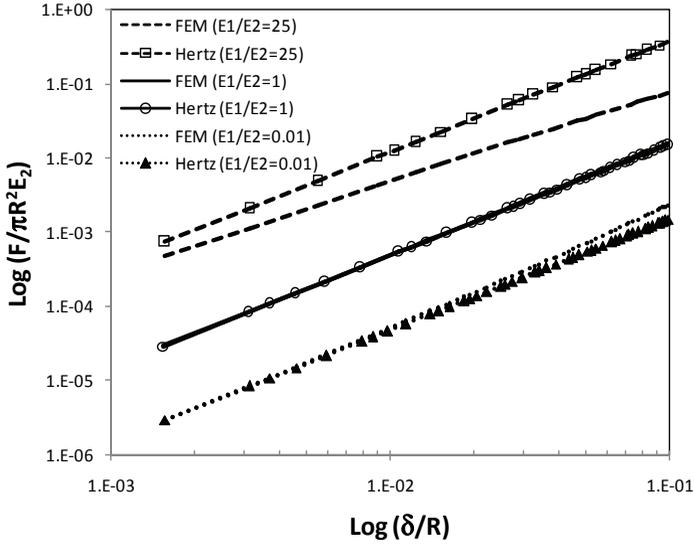
Figure 3: Comparisons of the finite element results and the Hertz contact theory in the indentation of film-substrate structures. As  $E_1/E_2=1$ , the film-substrate structure reduces to a homogeneous one.
