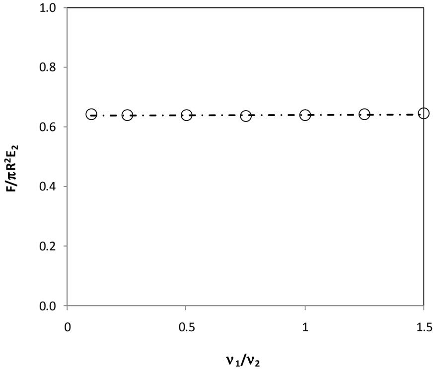
Figure 6: Maximum indentation load as a function of film Poisson's ratio.
