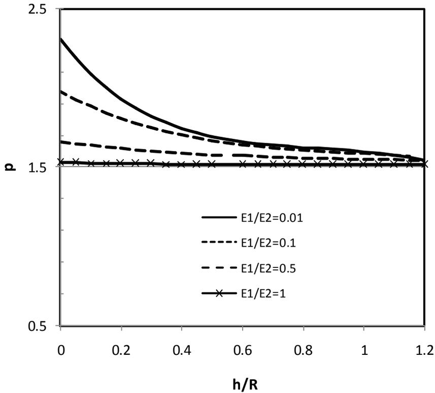
Figure 10: Variation of power coefficient,  $p$ , as a function of film thickness ( $h/R$ ).
