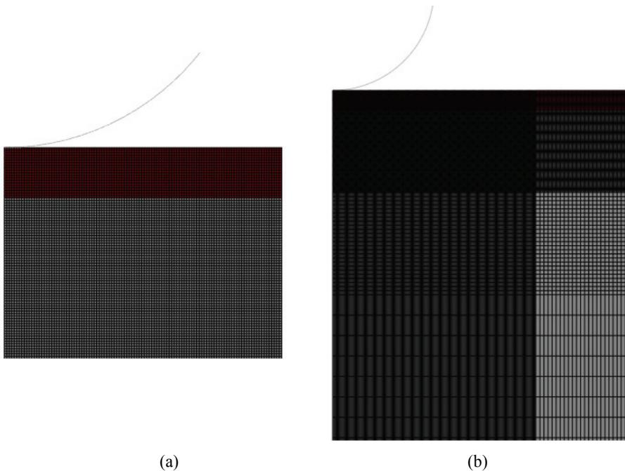
Figure 2: Finite element model of the spherical indentation of a film-substrate structure; (a) coarse mesh, (b) fine mesh.
