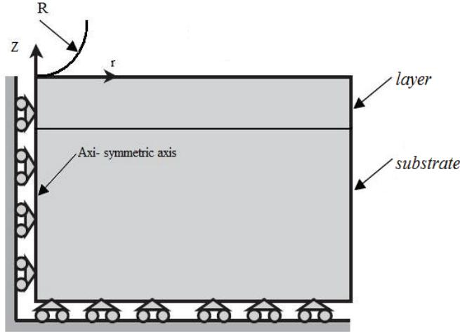
Figure 1: Schematic of the axisymmetric indentation of a semi-infinite film-substrate material with a rigid spherical indenter.
