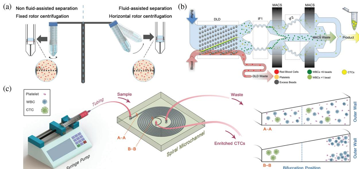
**FIGURE 3.** Schematic diagram of the microfluidic device for separating circulating tumor cells (CTC) in passive sorting. (a) Schematic diagram of a polydimethylsiloxane microfiltration membrane integrated microfluidic device for CTC capture (Han et al., 2022); (b) Schematic diagram of a deterministic lateral displacement microfluidic chip for CTC isolation (Fachin et al., 2017); (c) Schematic of the inertial sorting microfluidic chip for CTC separation (Kulasinghe et al., 2017).
