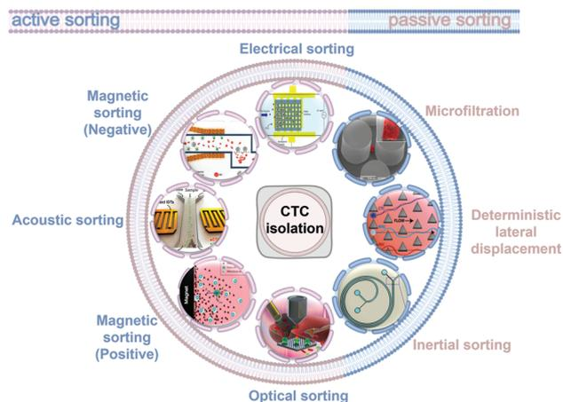
**FIGURE 1.** Summary of CTC isolation method including active sorting and passive sorting, where active sorting includes electric field sorting, magnetic field sorting, acoustic field sorting, and optical tweezers sorting. Passive sorting includes microfiltration, deterministic lateral displacement, and inertial sorting.
