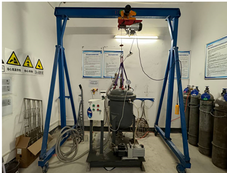
Figure 1: High-pressure carbonation reactor.
