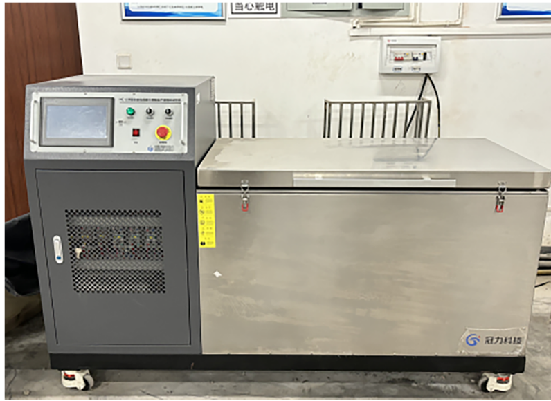
Figure 2: Experimental setup for sulfate wet-dry cycling of concrete specimens.
