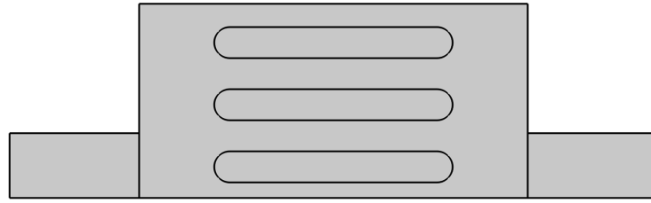
Figure 6: Plane cooling channels with three parallel fins.
