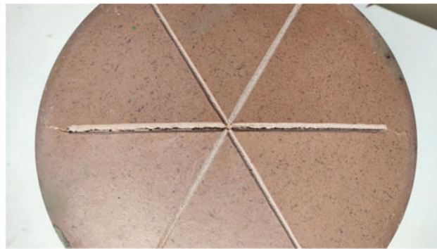
Figure 10: Fracture condition of the soft PSD after the monomial opening test
