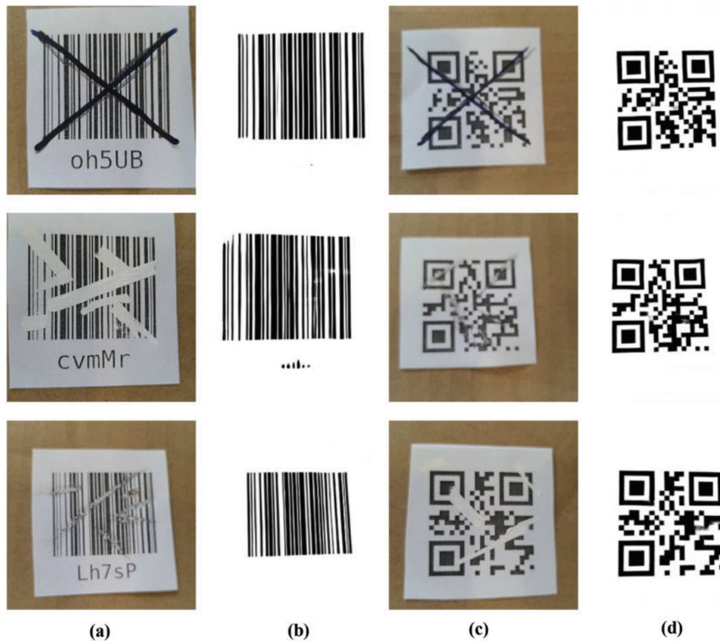
Figure 9: Real-time demonstration of 1D barcode and QR code restoration: (a) barcode input, (b) barcode restored, (c) QR code input, (d) QR code restored
