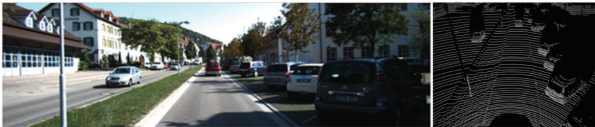
Figure 36: Example from the KITTI dataset: Left: RGB image, Right: Associated point cloud
