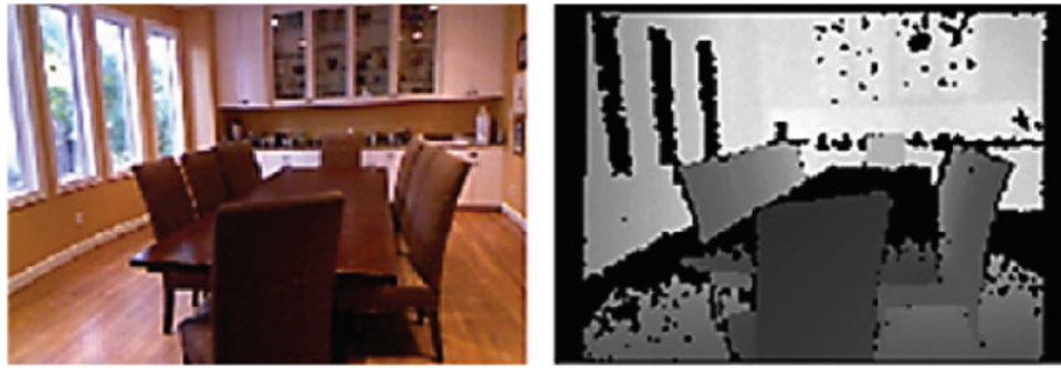
Figure 6: Example of data captured by an RGB-D camera: RGB image (left) and depth map (right) [32]
