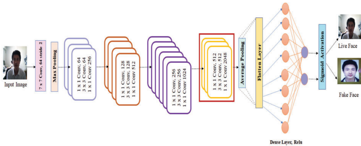
Figure 5: The modified ResNet-50 architecture highlights the red-marked region, representing the fine-tuned convolutional layers optimized for face liveness detection
