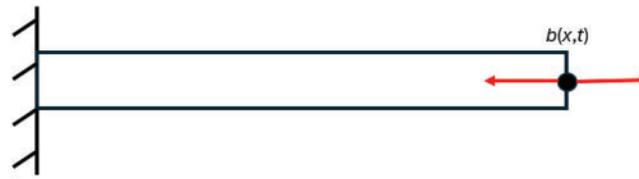
**Figure 6:** A damped system subjected to forced vibration
