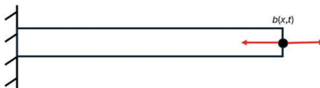
**Figure 9:** A rod subjected to a harmonic load at the free end without a damping effect
