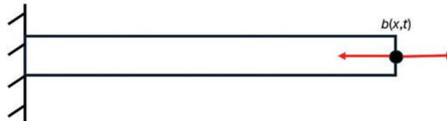
**Figure 4:** A bar that is initially at rest is subjected to a harmonic loading condition at the free end
