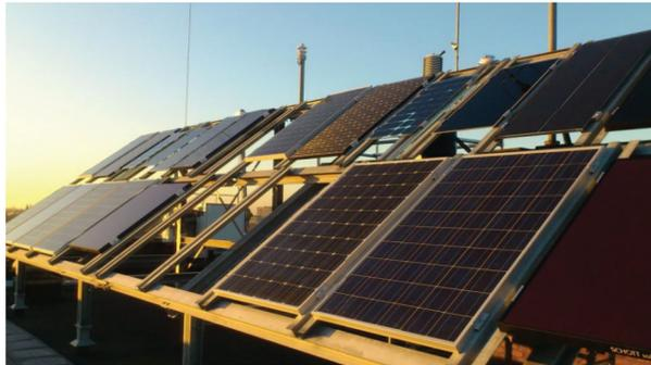
**Figure 3:** The Utrecht University Photovoltaic Outdoor Test (UPOT) facility measures the real-world performance of various commercial and prototype PV modules [38]
