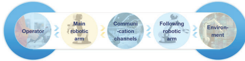
Figure 5: Force feedback bilateral remote operating system structure
