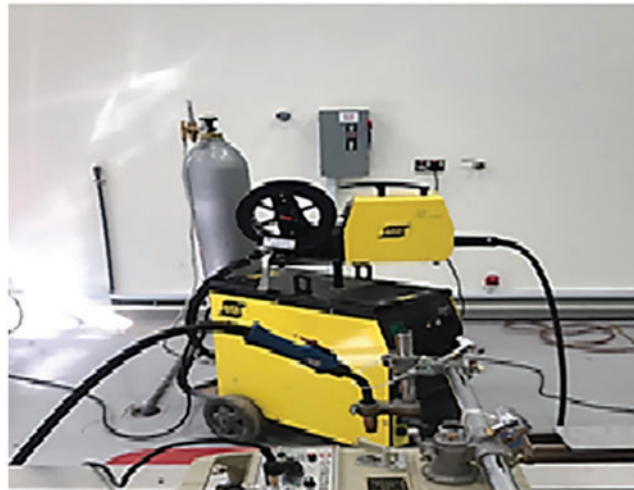
Figure 1: MIG welding machine with a motorized carriage
