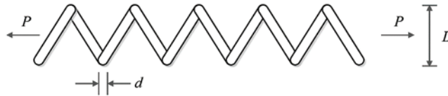
Figure 17: Schematic of the tension/compression spring design
