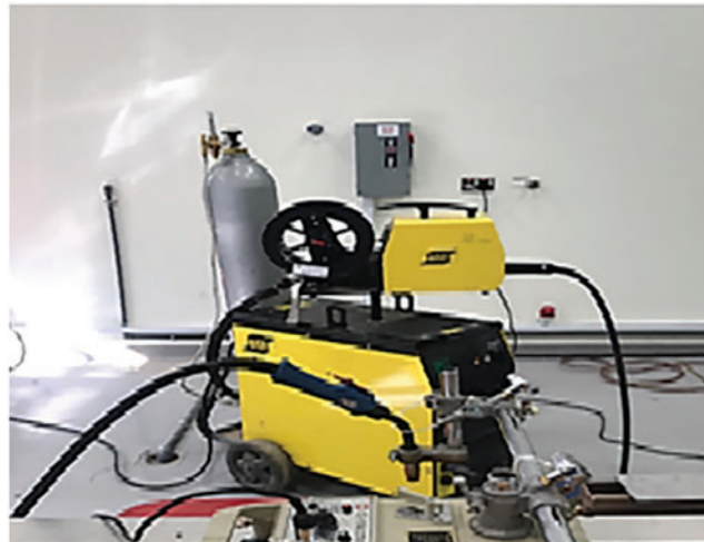
Figure 1: MIG welding machine with a motorized carriage
